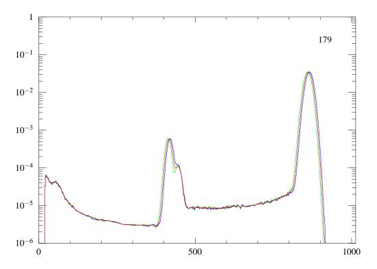
Green and blue is the tabulated response. Red is the interpolated response. This is an especially difficult situation when the fluorescence peak (on the right) "collides" with the escape peak (on the left). — Works well. (notice that the interpolation keeps the location of the fluorescence peak but shifts the escape peak appropriately).
