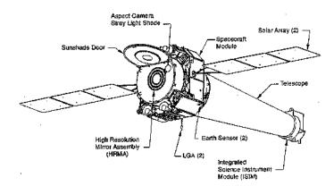
Figure 1.1: The *Chandra* Observatory with certain subsystems labeled. LGA is an acronym for the Low Gain Antenna.
