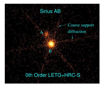
Figure 9.26: LETG/HRC-S zeroth order image of Sirius A and B. The two stars are separated by  $\sim 4''$ . Flux from Sirius A is due to the small but finite UV response of the detector. The star-shaped structure is due to coarse support diffraction.
