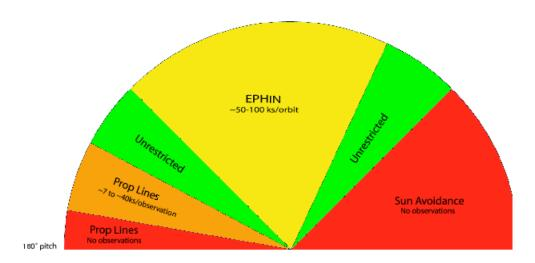
Figure 3.3: Diagram to illustrate ranges of solar pitch angle (the angle between the pointing direction and the satellite-Sun line) within which different observing limitations apply. Table 3.1 provides quantitative estimates for the observing limitations in the solar pitch angle ranges shown in the drawing.
