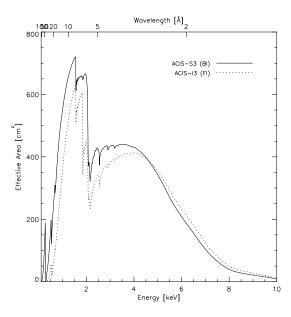
Figure 6.5: The **HRMA**/ACIS predicted effective area versus the energy on a linear scale. The dashed line is for the FI CCD I3, and the solid line is for the BI CCD S3.
