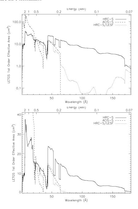
Figure 9.17: LETGS 1st-order effective area for an on-axis point source, with HRC-S, HRC-S LESF and ACIS-S detector configurations with log and linear scaling. Positive and negative orders are summed. LETG+ACIS-S areas were computed using an effective area model that included the effects of contamination build-up extrapolated to the level expected in mid-May 2008. Note that the vertical scale of the linear plot has been truncated.
