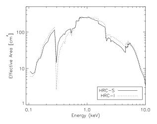
Figure 7.17: The effective area of the HRMA/HRC-I (dashed line) and the central segment of the HRMA/HRC-S in imaging mode (solid line) integrated over the full *PSF*. Absorption edges are due to the iridium coating of the telescope, the CsI MCP coating, and the polyimide/Al of the UVIS. The results of the low energy in-flight QE calibration have been incorporated into these curves.
