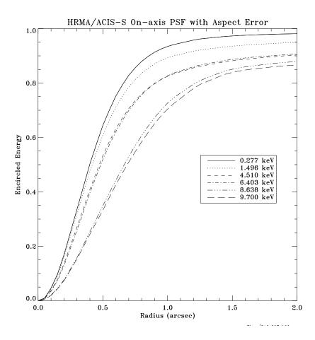
Figure 4.20: The fractional encircled energy as a function of angular radius expected for in flight ACIS-S(S3) measurements for an on-axis point-source at selected X-ray energies. The curves are the combined response of the four nested mirror pairs, typical aspect uncertainties, and the ACIS response function.
