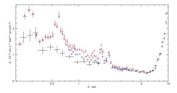
Figure 6.23: ACIS -S3 spectrum of the non-X-ray background (large crosses) overlaid on the quiescent blank sky spectrum. Small crosses show the total sky spectrum, while squares show the diffuse component left after the exclusion of all point sources detectable in this 90 ks exposure. Standard grade filtering and VF filtering are applied. The background and blank-sky spectra are normalized to the same flux in the 10-12 keV band.
