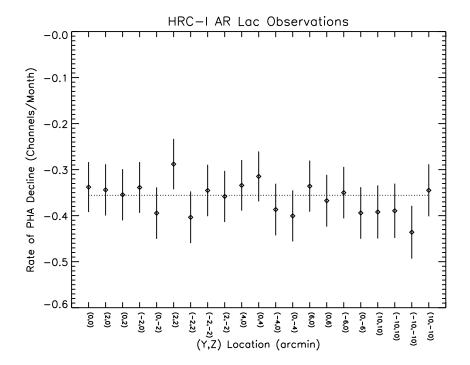
Figure 7.14: The rate of change of the median PHA derived for AR Lac observations carried out at numerous locations across the HRC-I detector, based on observations from Cycles 2-7. The PHA values are corrected for spatial variations separately for each set of observations. The dotted horizontal line represents the mean value of the gain drop.
