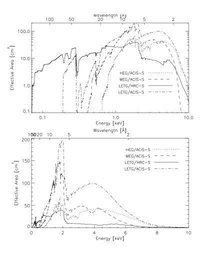
Figure 1.4: Comparison of the first-order effective areas in square centimeters (integrated over the line spread function) of the MEG, HEG and LETG spectrometers. The (+/-) first orders of the diffracted spectrum have been added.
