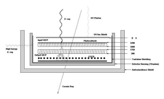
Figure 7.3: A schematic of the HRC Micro-channel-Plate detector.
