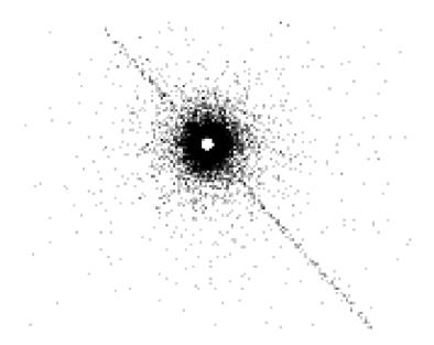
Figure 6.14: Trailed image of a strong X-ray source. The core of the image is faint due to pileup. Most events here are rejected because of bad grades. The readout direction is parallel to the trail.
