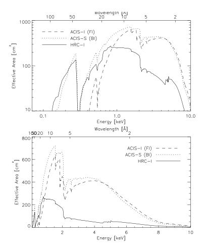
Figure 1.3: Comparison of the on-axis effective areas for observing a point sourc(integrated over the PSF) of the HRMAHRC-I, the HRMA/ACIS(FI), and the HRMA/ACIS(BI) combinations. The ACIS curves show the predicted values for the middle of Cycle 9 (2008-05-15).
