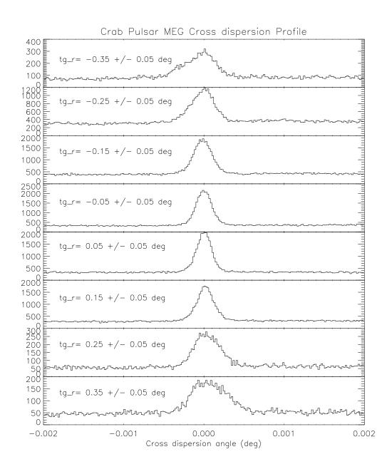
Figure 8.19: The cross dispersion profile is shown for eight slices of the dispersed MEG spectrum of the Crab pulsar. There is an asymmetry caused by misaligned gratings that becomes most evident at large dispersion.
