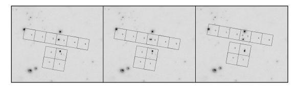
Figure 3.1: Examples of offset pointing with ACIS. North is up and East is to the left. Roll is measured positive, West of North. The roll angle shown is 10°. Left Panel: The target, a bright x-ray source, is centered at the nominal ACIS-S aimpoint. Middle Panel: The target is offset with (Y,Z) offset of (-1,0) arcmin. In the Right Panel the offset is (-1,-3). Note the small circle at the location of the ACIS-S aimpoint.
