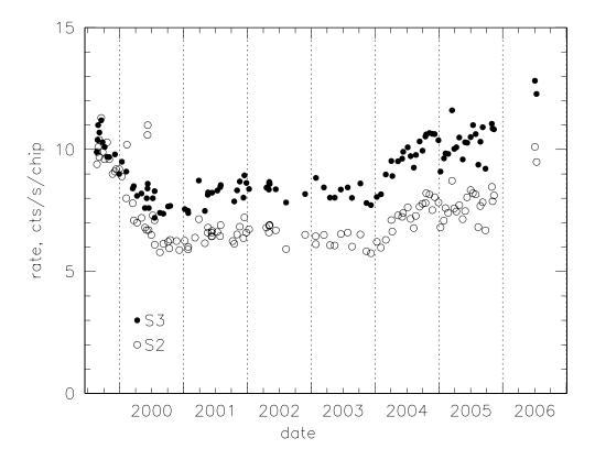
Figure 6.24: Total telemetered background rates (including all grades and the standard upper event cutoff at  $15~{\rm kev}$ ) for chips S2 (FI) and S3 (BI) as a function of time. Vertical dashed lines are year boundaries.
