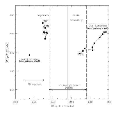
Figure 6.12: Position of the optical axis on the S3 CCD at various times in the mission. In 1999, the optical axis was at (229,531) and an offset was used to place the aimpoint on node 1 of the CCD at (293,519). By 2005, the optical axis had drifted to (231,526) and the aimpoint was offset by -20" in Y to 276,497). In this case, dither will move the image across the node boundary. Currently, the standard offset is +10" placing the aimpoint on node 0 of the CCD at (215,497).
