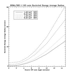
Figure 7.6: Encircled energy as a function of source off-axis angle for 50% and 90% encircled energy for 1.49 and 6.40 keV for the combined  $\mathbf{HRMA}/\mathrm{HRC}$ -I. A conservative contribution from the aspect solution is included (FWHM = 20  $\mu$ m (0.41")). A plot for the combined  $\mathbf{HRMA}/\mathrm{HRC}$ -S would be almost identical since the PSFs of the two instruments are virtually identical and independent of off-axis angle.
