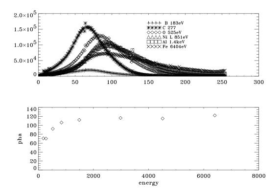
Figure 7.7: The pulse height versus energy for the HRC-I detector and the centroid of the pulse height distribution versus energy. This data set was obtained at SAO during flat field, normal-incidence-illumination tests. The voltage settings have been changed in-flight and thus the applicability of these data is questionable and they are presented here for purposes of illustration only.
