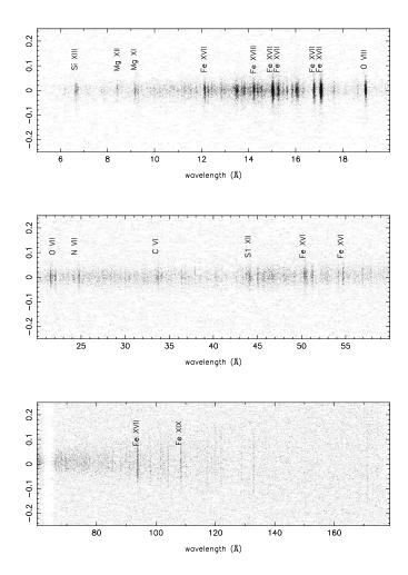
Figure 9.24: HRC-S detector image of a Capella observation, showing positive order dispersion. Both axes are in Å with 1.148 Å/mm. The increasing cross-dispersion extent of lines at longer wavelengths is due to a stigmatism in the HRMA/LETG system. The positive-order HRC-S plate gap is at  $\sim63~\mbox{Å}.$
