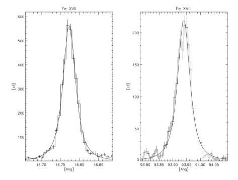
Figure 9.9: LETGS line response function as illustrated by two bright Fe lines (Fe XVII at  $\sim 17$  Å and Fe XVIII at  $\sim 94$  Å) using in-flight calibration observations of Capella. The solid curves are best-fit Moffat functions with  $\beta = 2.5$ .
