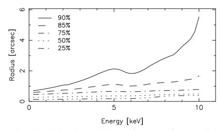
Figure 4.7: The radii of selected encircled energy fractions as functions of X-ray energy for an on-axis point source, calculated from the mirror model derived from ground-based calibration data.
