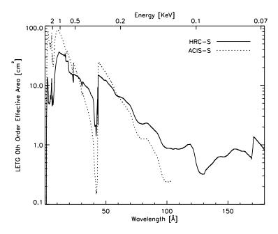
Figure 9.16: LETGS 0th-order effective area for an on-axis point source for the LETG with HRC-S and ACIS-S detectors. The 0th-order effective area for the HRC-S/LESF combination is the same as for the HRC-S. LETG+ACIS-S areas were computed using an effective area model that included the effects of contamination build-up extrapolated to the level expected in mid-May 2008.
