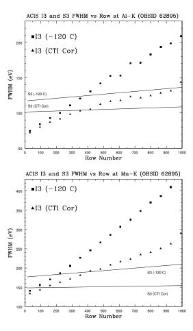
Figure 6.9: An example of the application of the *CXC* CTI-corrector in two energy bands. The upper plot shows data for the Al-K line, and the lower for Mn-K. The square data points are the FWHM of lines averaged over 32-row bins. The triangle data points are the FWHM of CTI-corrected lines. The upper line shows the uncorrected performance of the S3 chip, while the lower line shows the CTI-corrected performance of the S3 chip. These data are from March 2000.
