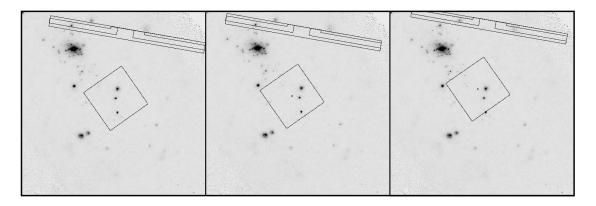
Figure 3.2: Example of offset pointing with HRC. North is up and East is to the left. Roll is measured positive, West of North. The roll angle shown is 10°. Left Panel: The target, the middle source in a group of three aligned N-S, is at the nominal HRC-I aimpoint. Center Panel: The target is offset with (Y,Z) offset of (-5,0) arcmin. Right Panel: The offset is (-5,-5). Note the small dot at the location of the HRC-I aimpoint.
