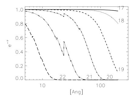
Figure 9.27: The ISM transmittance within the LETGS bandpass for different values of neutral hydrogen column density  $10^{17}$ - $10^{22}$  cm<sup>2</sup>.
