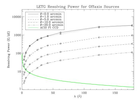
Figure 9.12: LETG spectral resolving power for off-axis sources. The predicted LETG resolving power  $(E/\Delta E)$  is shown versus wavelength for various off-axis distances. For comparison, the spectral resolution for ACIS front-illuminated CCD chips is shown. Note that the ACIS/FI curve does not include the effects of CTI, which progressively degrades resolution away from the readout edge.
