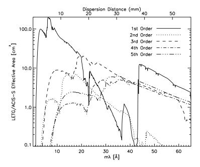
Figure 9.20: The combined HRMA/LETG/ACIS-S effective areas for 1st and higher orders. LETG+ACIS-S areas were computed using an effective area model that included the effects of contamination build-up extrapolated to the level expected in mid-May 2008. Positive and negative orders are summed. (LETG efficiencies for orders 2,4,5,6,7 were updated in August 2004 in CALDB 2.28.)
