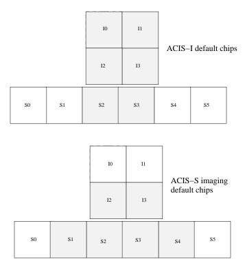
Figure 6.2: A schematic drawing of the ACIS focal plane, not to scale. The ACIS-I array consists of chips I0-I3. Chips S2 and S3 are often turned in addition to I0-I3 when ACIS-I is used in imaging mode as indicated in the top figure. ACIS-S consists of chips S0-S5. When operated in imaging mode chips S1-S4 plus I2 and I3 are often turned on (bottom figure). When operated in spectroscopy mode S0-S5 are usually turned on. See 6.19.1 for more details on chip choices.
