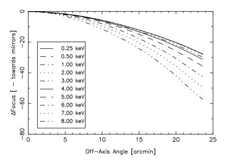
Figure 4.11: The HRMA focal surface (from simulations), indicating its dependence on energy and off-axis source position. It deviates more from the detector planes at higher energies and larger off-axis angles, leading to significant degradation of image quality.
