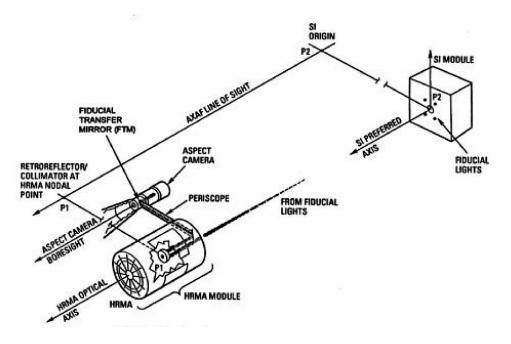
Figure 5.3: Fiducial Transfer System
