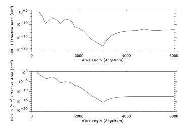
Figure 7.16: The HRC-I (top) and the center section of the HRC-S (bottom) UV/Ion shield effective area as a function of wavelength.
