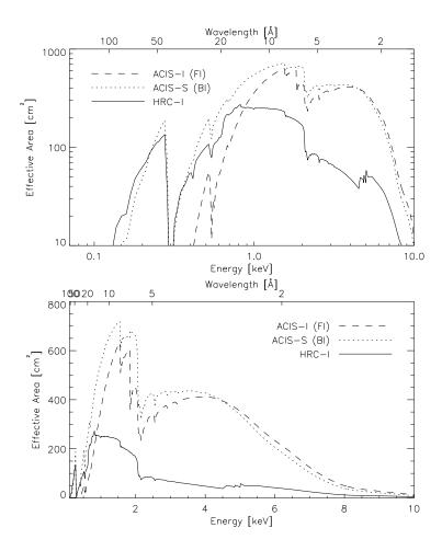
Figure 1.3: Comparison of the on-axis effective areas for observing a point source (integrated over the *PSF*) of the **HRMA/HRC-I**, the **HRMA/ACIS(FI)**, and the **HRMA/ACIS(BI)** combinations. The ACIS curves show the predicted values for the middle of Cycle 8 (2007-05-15).
