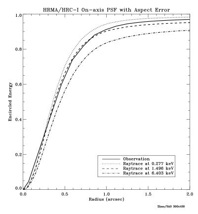
Figure 7.5: The predicted and observed fractional encircled energy as a function of radius for an on-axis point source observed with the **HRMA/HRC-I**. The calculations (at two energies, 0.277 keV and 6.40 keV) include a very conservative estimate of the aspect solution (FWHM = 20  $\mu$ m (0.41")). Flight data from an observation of AR Lac are also shown.
