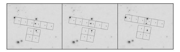
Figure 3.1: Examples of offset pointing with ACIS. North is up and East is to the left. Roll is measured positive, West of North. The roll angle shown is 10°. Left Panel: The target, a bright x-ray source, is centered at the aimpoint. Middle Panel: The target is offset from the ACIS-S nominal aimpoint with (Y,Z) offset of (-1,0) arcmin. In the Right Panel the offset is (-1,-3). Note the small circle at the location of the ACIS-S aimpoint.
