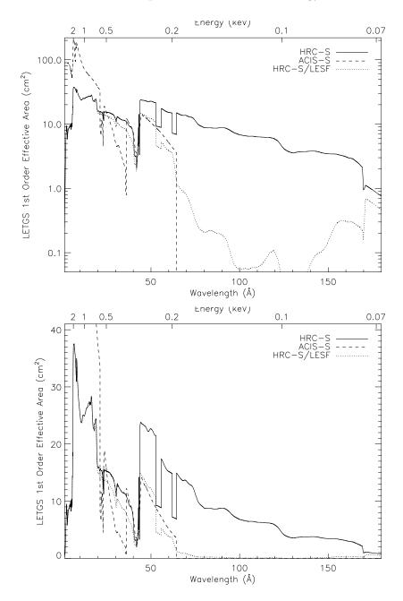
Figure 9.17: LETGS 1st-order effective area for an on-axis point source, with HRC-S, HRC-S LESF and ACIS-S detector configurations with log and linear scaling. Positive and negative orders are summed. LETG+ACIS-S areas were computed using an effective area model that included the effects of contamination build-up extrapolated to the level expected in mid-May 2007. Note that the vertical scale of the linear plot has been truncated.
