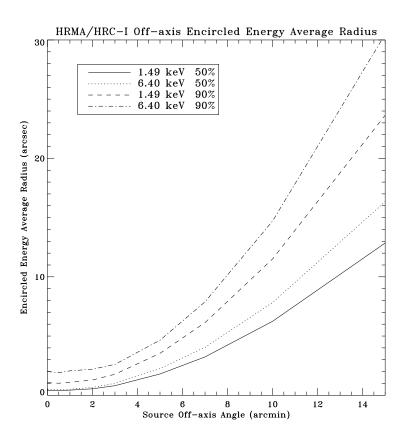
Figure 7.6: Encircled energy as a function of source off-axis angle for 50% and 90% encircled energy for 1.49 and 6.40 keV for the combined  $\mathbf{HRMA}/\mathrm{HRC}$ -I. A conservative contribution from the aspect solution is included (FWHM = 20  $\mu$ m (0.41")). A plot for the combined  $\mathbf{HRMA}/\mathrm{HRC}$ -S would be almost identical since the PSFs of the two instruments are virtually identical and independent of off-axis angle.
