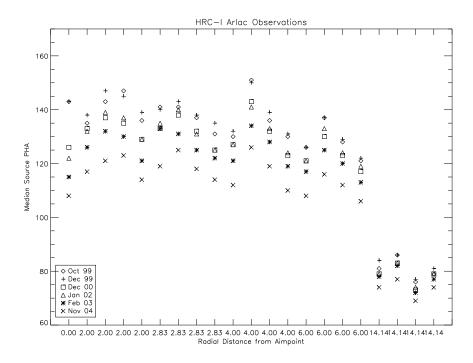
Figure 7.12: The median PHA derived for AR Lac observations carried out at numerous locations across the HRC-I detector. There also exist intrinsic variations in the spectrum which have not been accounted for in this figure.
