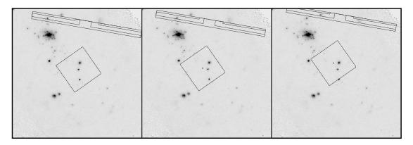
Figure 3.3: Example of offset pointing with HRC. North is up and East is to the left. Roll is measured positive, West of North. The roll angle shown is 10°. Left Panel: The target, the middle source in a group of three aligned N-S, is centered. Center Panel: The target is offset from the HRC-I nominal aimpoint with (Y,Z) offset of (-5,0) arcmin. Right Panel: The offset is (-5,-5). Note the small dot at the location of the HRC-I aimpoint.
