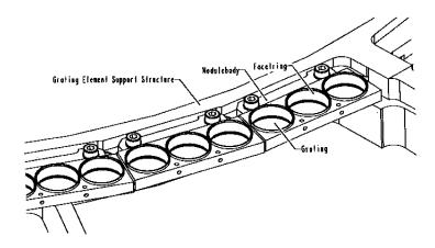
Figure 9.3: A closeup view of the LETG GESS showing two complete grating modules. Each module has three holes that hold the arrays of grating facets.
