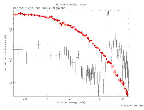
Figure 6.27: Spectra of different background flares in chip S3. Thick crosses show a common flare species that affects only the BI chips. Thin crosses show one of the several less common flare species that affect both the BI and FI chips. Note how both these spectra are different from the quiescent spectrum (see Figure 6.21).
