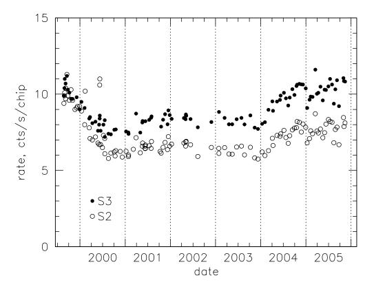
Figure 6.24: Total telemetered background rates (including all grades and the standard upper event cutoff at 15 kev) for chips S2 (FI) and S3 (BI) as a function of time. Vertical dashed lines are year boundaries.
