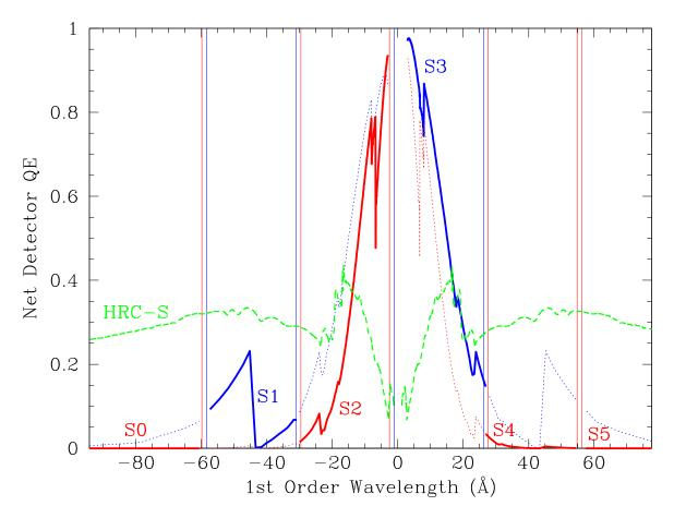
Figure 9.6: Comparison of HRC-S and ACIS-S QEs (updated for AO8) when used with the LETG. (Y-offset = 0 for HRC-S, +1.5' for ACIS-S). Dashed (green) line is for HRC-S, thick solid curves are for ACIS (updated for ACIS effective area degradation). Y-offsets may be chosen to tailor the coverage of BI chips (S1 and S3; top/blue QE curve) and FI chips (S0,S2,S4,S5; bottom/red curve). Vertical lines indicate ACIS chip gaps (with dither, 1.5 Å). For clarity, -3 to +3 Å is not shown for ACIS.
