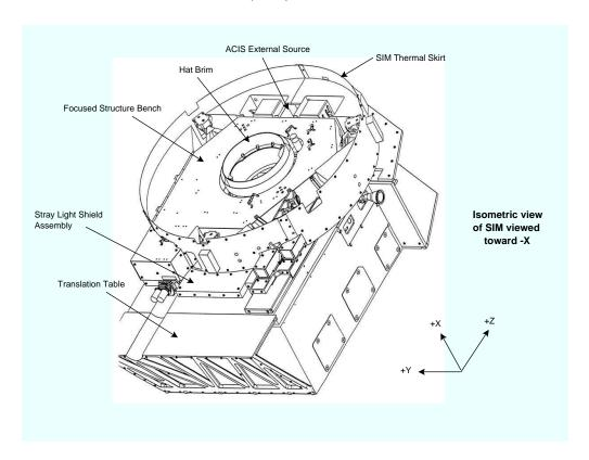
Figure 2.2: A schematic of the Science Instrument Module.
