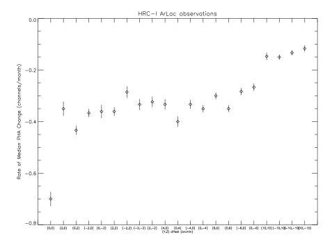
Figure 7.14: The rate of change of the median PHA derived for AR Lac observations carried out at numerous locations across the HRC-I detector.
