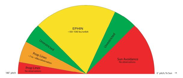
Figure 3.2: Diagram to illustrate ranges of solar pitch angle (the angle between the pointing direction and the satellite-Sun line) within which different observing limitations apply. Table 3.1 provides quantitative estimates for the observing limitations in the solar pitch angle ranges shown in the drawing.
