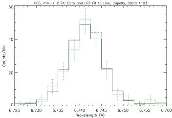
Figure 8.16: Representative Line Response Functions at two wavelengths for the HEG; 15 Å top, 6.7 Å bottom. Two of the bright lines in the HEG counterpart to the MEG Capella spectrum shown in Figure 8.2 have been fit by the instrumental LRF. The LRF is encoded in the HEG RMF created using CXC software and calibration parameters (mkgrmf, lsfparmN0003.)
