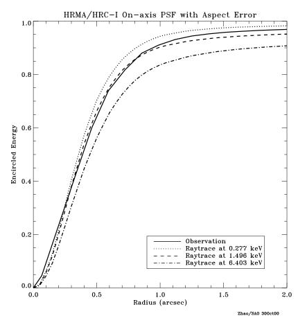
Figure 4.18: The HRMA/HRC-I on-axis fractional encircled energy as a function of angular radius from a point source (Ar Lac) observed in flight compared to raytrace simulations for an on-axis point-source at selected X-ray energies, including the aspect uncertainties and the HRC-I pixelization effects.
