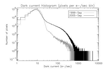
Figure 5.6: Differential histogram of dark current distribution for the ACA CCD in 1999-Aug (gray) and 2005-Sep (black)
