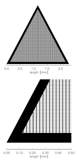
Figure 9.4: LETG facet structure schematic showing the basic shape of the individual grating elements and the relative sizes of the support structures. The upper view shows the entire facet, which comprises the triangular coarse support, the vertical fine supporting bars, and the (horizontal) grating bars. The grating bars themselves are not shown to scale. In the upper view every  $50^{\rm th}$  grating bar is drawn, in the lower view every  $10^{\rm th}$  bar.
