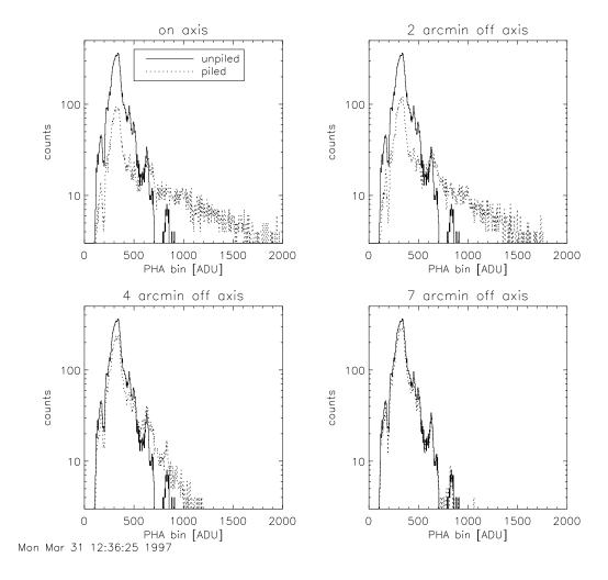
Figure 6.18: MARX simulations of the effect of pileup on the shape of the spectrum. The true (solid line) and the detected (dotted line) spectra are shown for four different viewing angles. The corresponding "pileup fractions" - see Section 6.14.2 - are 46%, 40%, 15%, and 2% as the image is moved progressively further off-axis. (Source: J. Kastner and M. Wise, CXC)
