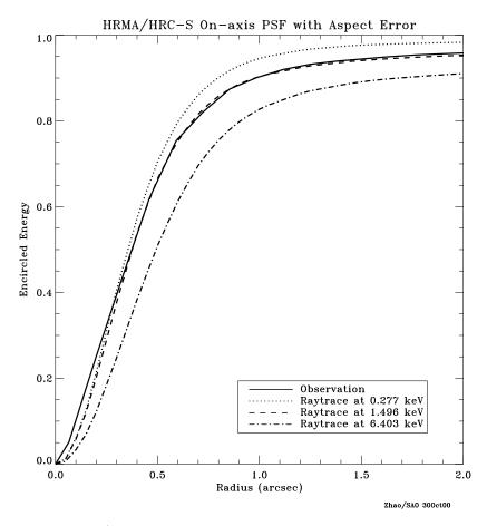
Figure 4.19: The HRMA/HRC-S on-axis fractional encircled energy as a function of angular radius from a point source (LMC X-1) observed in flight compared to raytrace simulations for an on-axis point-source at selected X-ray energies, including the aspect uncertainties and the HRC-S pixelization effects.
