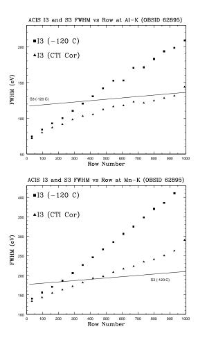
Figure 6.11: An example of the application of the *CXC* CTI-corrector in two energy bands. The first plot shows data for the Al-K line, and the second for Mn-K. The square data points are the FWHM of lines accumulated in 32-row bins. The triangle data points are the FWHM of CTI-corrected lines accumulated in 32-row bins. The line shows the nominal performance of the S3 chip. These data are from March 2000.
