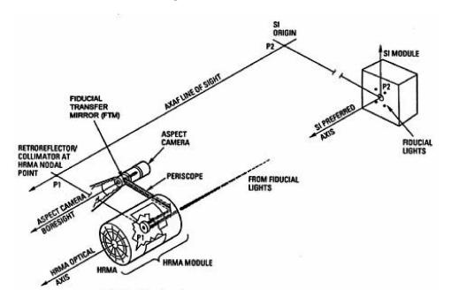
Figure 5.3: Fiducial Transfer System
