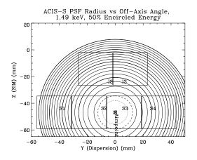
Figure 6.9: Approximate contours of constant 50% encircled energy at 1.49 keV when the ACIS-S default aimpoint is selected. The dotted line is 1 arcsec, the dashed line is 1.5 arcsec. The remainder are 1 arcsec intervals. The thicker solid lines highlight the 5, 10, 15 and 20 arcsec contours.
