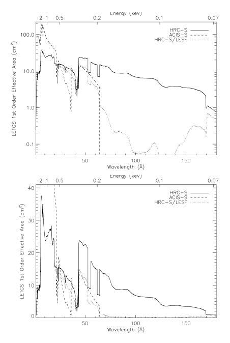
Figure 9.17: LETGS 1st-order effective area for an on-axis point source, with HRC-S, HRC-S LESF and ACIS-S detector configurations with log and linear scaling. Positive and negative orders are summed. LETG+ACIS-S areas were computed using an effective area model that included the effects of contamination build-up extrapolated to the level expected in mid-May 2006. Note that the vertical scale of the linear plot has been truncated.
