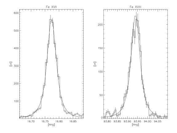
Figure 9.9: LETGS line response function as illustrated by two bright Fe lines (Fe XVII at ~ 17 Å and Fe XVIII at ~ 94 Å) using in-flight calibration observations of Capella. The solid curves are best fit beta models ( $\beta = 2.5$ ).
