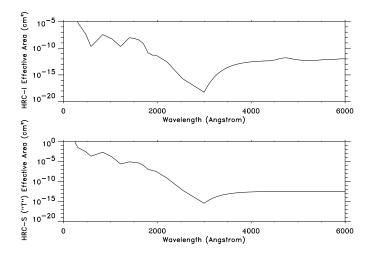
Figure 7.8: The HRC-I (top) and the center section of the HRC-S (bottom) UV/Ion shield effective area as a function of wavelength.
