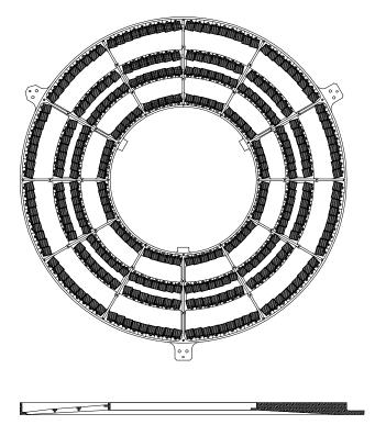
Figure 8.5: An (upper) front and side (lower) view of the HETG support structure (HESS). The grating facets are mounted to intercept the X-rays as they exit the HRMA; the front view is from the HRMA i.e., what an approaching X-ray would see. In the side view, the left cross-section shows that the four support rings are in different planes due to the Rowland curvature. The right cross-section is through a radial rib at one of the three mounting "ears".
