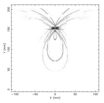
HRMA Off-axis Image & Ghost Rays 1.4967 keV Source: Azimuth = 0 arcmin Elevation = 53 arcmin
