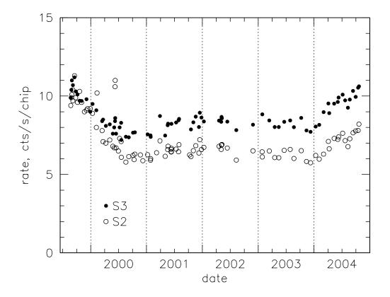
Figure 6.23: Total telemetered background rates (including all grades and the standard upper event cutoff at 15 kev) for chips S2 (FI) and S3 (BI) as a function of time. Vertical dashed lines are year boundaries.
