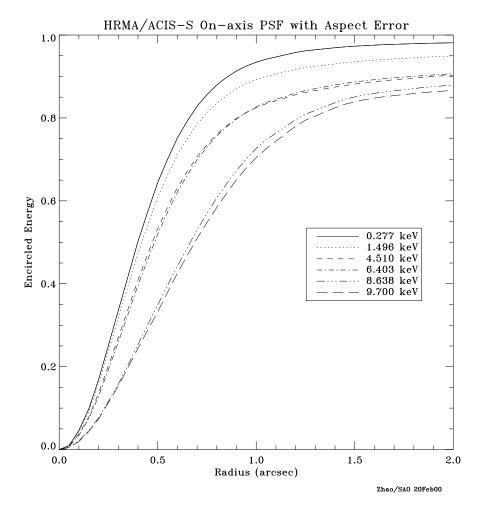
Figure 4.17: The fractional encircled energy as a function of angular radius expected for in flight ACIS-S(S3) measurements for an on-axis point-source at selected X-ray energies. The curves are the combined response of the four nested mirror pairs, typical aspect uncertainties, and the ACIS response function.
