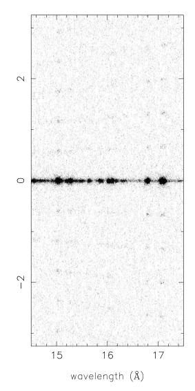
Figure 9.23: Detail of Figure 9.22, showing the LETG/HRC-S image of bright lines in Capella. Both axes are in Å with 1.148 Å/mm. The Fe XVII lines at  $\sim 15$  and 17 Å are the brightest in the LETG Capella spectrum. Faint features above and below the primary spectrum are due to fine support structure diffraction.
