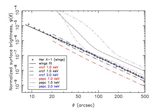
Figure 4.8: Radial profile of the Her X-1 scattering wings for 1.0-2.0 keV. The heavy solid line is a powerlaw plus exponential cutoff fit to the data; the heavy dash-dot lines are results from an empirical model based on ground testing for 1.0, 1.5, and 2.0 keV (lower curve to upper curve). The light lines are the ROSAT PSPC profile evaluated using the parameterization of Boese 2000.
