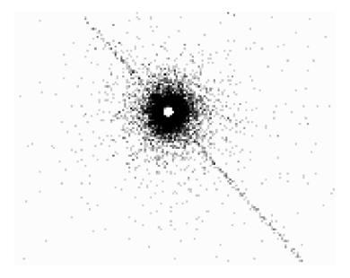
Figure 6.13: Trailed image of a strong X-ray source. The core of the image is faint due to pileup. Most events here are rejected because of bad grades. The readout direction is parallel to the trail.
