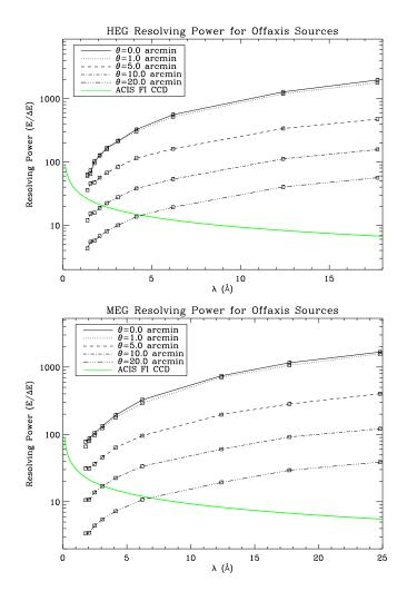
Figure 8.23: The effects of off-axis pointing on the HETG grating spectral resolution. Using MARX, we have simulated an observation of a point source at increasing off-axis positions. The effect on the resolving power  $(E/\Delta E)$  is shown as a function of photon energy for off-axis angles of 0', 1', 5', 10', and 20'. The spectral resolution of an ACIS Front Illuminated (FI) CCD at a point near the framestore region is shown for comparison.
