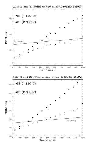
Figure 6.11: An example of the application of the *CXC* CTI-corrector in two energy bands. The first plot shows data for the Al-K line, and the second for Mn-K. The square data points are the FWHM of lines accumulated in 32-row bins. The triangle data points are the FWHM of CTI-corrected lines accumulated in 32-row bins. The line shows the nominal performance of the S3 chip. This data is from March 2000.
