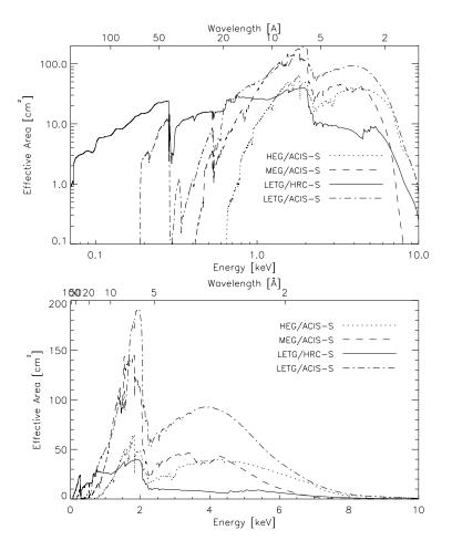
Figure 1.4: Comparison of the first-order effective areas in square centimeters (integrated over the line spread function) of the MEG and HEG and LETG spectrometers. The (+/-) first orders of the diffracted spectrum have been added.
