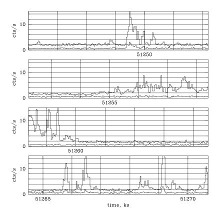
Figure 6.24: An example of the ACIS background counting rate versus time - BI chip (S3; top curve) and an FI chip (I2; bottom curve). These are for the standard grades and the band from 0.3 - 10 keV.
