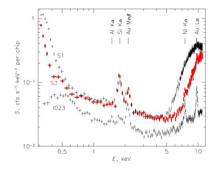
Figure 6.20: Energy spectra of the charged particle ACIS background with ACIS in the stowed position (a 50 ks exposure taken in September 2002; standard grade filtering, no VF filtering). Line features are due to fluorescence of material in the telescope and focal plane.
