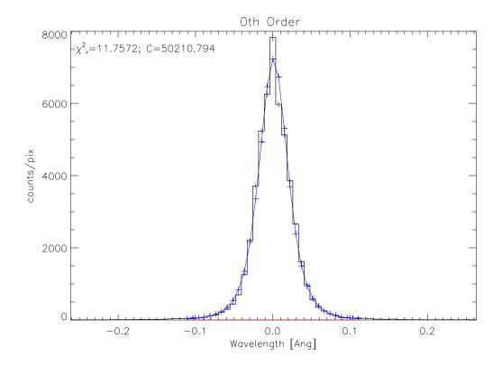
Figure 9.8: Observed LETG zeroth-order LRF from in-flight calibration observations of the active late-type binary Capella. The model profile, the continuous curve, is a beta model (see text) corresponding to the best fit value of  $\beta = 2.5$ . The reduced  $\chi^2$  of 11.8 certainly indicates a statistically poor fit to these very high S/N data, but the beta model is a good approximation to the LRF for weaker dispersed lines.
