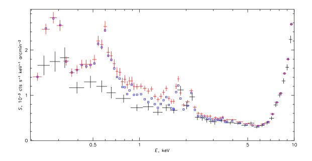
Figure 6.22: ACIS -S3 spectrum of the non-X-ray background (large crosses) overlaid on the quiescent blank sky spectrum. Small crosses show the total sky spectrum, while squares show the diffuse component left after the exclusion of all point sources detectable in this 90 ks exposure. Standard grade filtering and VF filtering are applied. The background and blank-sky spectra are normalized to the same flux in the 10-12 keV band.
