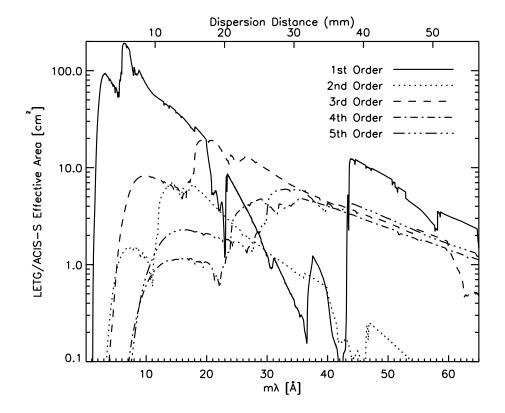
Figure 9.20: The combined HRMA/LETG/ACIS-S effective areas for first and higher orders. LETG+ACIS-S areas were computed using an effective area model that included the effects of contamination build-up extrapolated to the level expected in mid-May 2006. Positive and negative orders are summed. (Efficiencies for orders 2,4,5,6,7 were updated in August 2004 in CALDB 2.28.)
