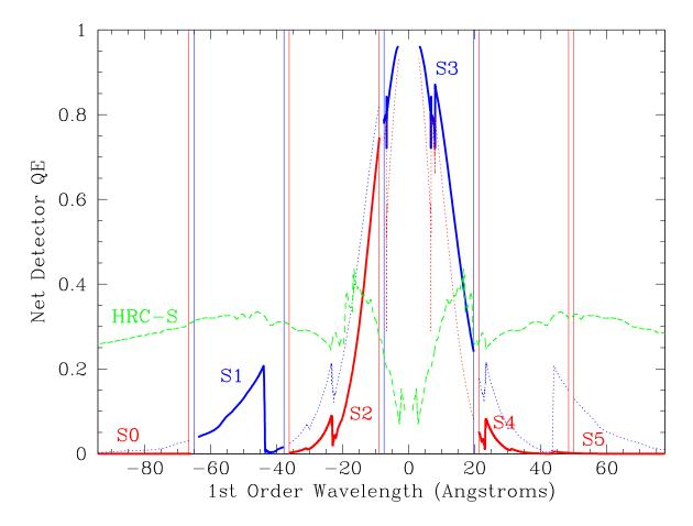
Figure 9.6: Comparison of HRC-S and ACIS-S QEs when used with the LETG. (Y-offset = 0 for HRC-S, -0.33' for ACIS-S). Dashed (green) line is for HRC-S, thick solid curves are for ACIS (updated for ACIS effective area degradation). Y-offsets may be chosen to tailor the coverage of BI chips (S1 and S3; top/blue QE curve) and FI chips (S0,S2,S4,S5; bottom/red curve). Vertical lines indicate ACIS chip gaps (with dither, 1.5 Å). For clarity, -3 to +3 Å is not shown for ACIS.
