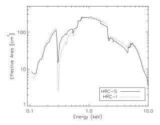
Figure 7.9: The effective area of the **HRMA**/HRC-I (dashed line) and the central segment of the **HRMA**/HRC-S in imaging mode (solid line) integrated over the full PSF. Absorption edges are due to the iridium coating of the telescope, the CsI MCP coating, and the polyimide/Al of the UVIS. The results of the low energy in-flight QE calibration have been incorporated into these curves.
