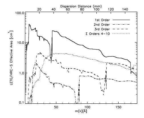
Figure 9.18: The combined HRMA/LETG/HRC-S effective area, illustrating the relative strengths of 1st and higher orders. Positive and negative orders are summed. In the label for the bottom axis, m is the order number. See the text for an example of how to determine the relative strength of overlapping lines from different orders. (Efficiencies for orders 2,4,5,6,7 were updated in August 2004 in CALDB 2.28.)
