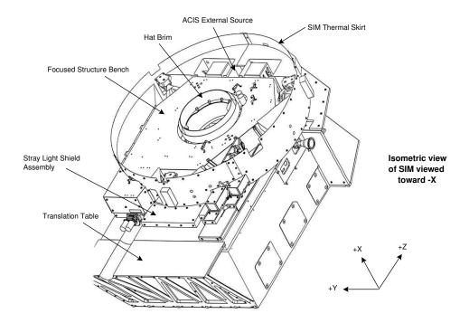
Figure 2.2: A schematic of the Science Instrument Module.
