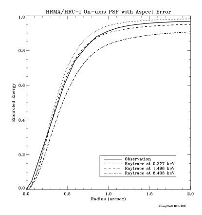
Figure 7.5: The predicted and observed fractional encircled energy as a function of radius for an on-axis point source observed with the **HRMA**/HRC-I. The calculations (at two energies, 0.277 keV and 6.40 keV) include a very conservative estimate of the aspect solution (FWHM = 20  $\mu$ m (0.41")). Flight data from an observation of AR Lac are also shown.
