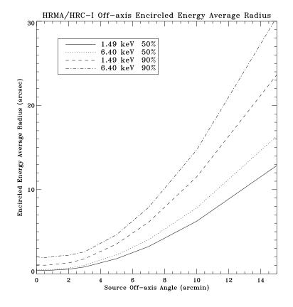
Figure 7.6: Encircled energy as a function of source off-axis angle for 50% and 90% encircled energy for 1.49 and 6.40 keV for the combined **HRMA**/HRC-I. A conservative contribution from the aspect solution is included (FWHM = 20  $\mu$ m (0.41")). A plot for the combined **HRMA**/HRC-S would be almost identical since the PSFs of the two instruments are virtually identical and independent of off-axis angle.
