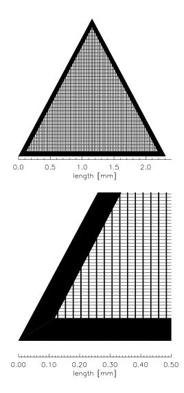
Figure 9.4: LETG facet structure schematic showing the basic shape of the individual grating elements and the relative sizes of the support structures. The upper view shows the entire facet, which comprises the triangular coarse support, the vertical fine supporting bars, and the (horizontal) grating bars. The grating bars themselves are not shown to scale. In the upper view every 50<sup>th</sup> grating bar is drawn, in the lower view every 10<sup>th</sup> bar.
