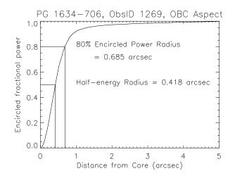
Figure 6.7: The on-orbit encircled broad-band energy versus radius for an ACIS observation of point source PG1634-706. The effective energy is 1 keV.
