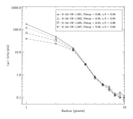
Figure 6.16: The effects of pileup on the radial distribution of the PSF are illustrated. These data were taken during ground calibration at the XRCF. The specific "OBSIDs", the counting rate per CCD frame ("c/f"), and the "pileup fraction" as defined in Section 6.14.2 are given in the inset.
