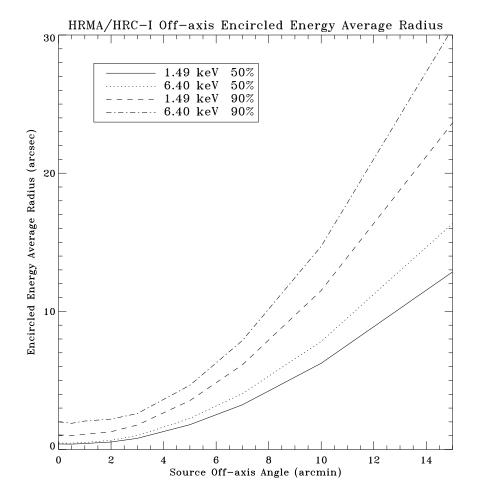
Figure 4.11: **HRMA**/HRC-I encircled energy average radii for circles enclosing 50% and 90% of the power at 1.49 and 6.40 keV as a function of off-axis angle. The HRC-I surface is a flat plane perpendicular to the optical axis, which does not follow the curved *Chandra* focal plane. These curves include the blurs due to the HRC-I spatial resolution and the *Chandra* aspect error.
