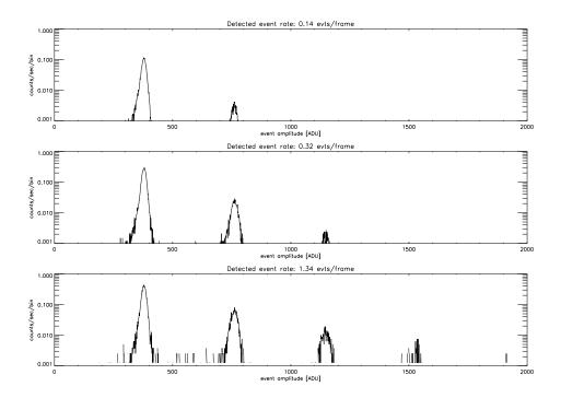
Figure 6.15: The effects of pileup at 1.49 keV (Al K $\alpha$ ) as a function of source intensity. Data were taken during HRMA-ACIS system level calibration at the XRCF. Single-photon events are concentrated near the pulse height corresponding to the Al K $\alpha$  line (~ 380 ADU), and events with 2 or more photons appear at integral multiples of the line energy.
