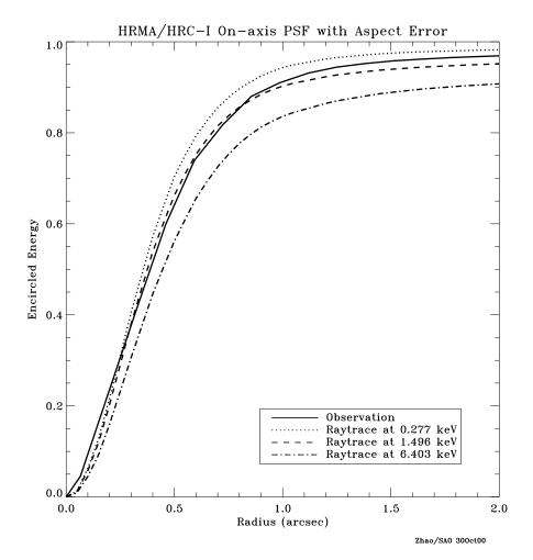
Figure 4.15: The fractional encircled energy as a function of angular radius observed in flight compared to model calculations for an on-axis point-source at selected X-ray energies. The curves are the combined response of the four nested mirror pairs, typical aspect uncertainties, and the HRC-I response function.
