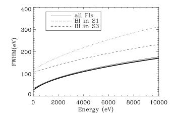
Figure 6.10: The ACIS pre-launch energy resolution as a function of energy. (Source: CXC Calibration group).
