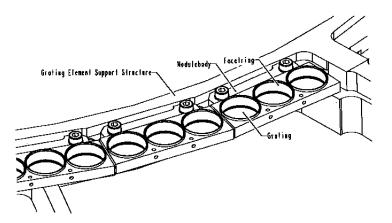
Figure 9.3: A closeup view of the LETG GESS showing two complete grating modules. Each module has three holes which hold the arrays of grating facets.
