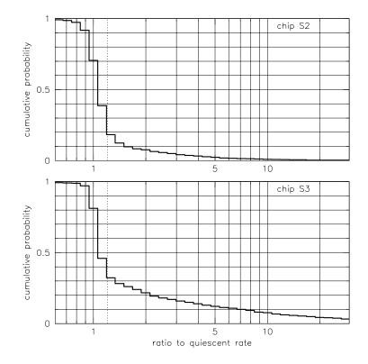
Figure 6.25: An estimate of the cumulative probability that the ratio of the background counting rate to the quiescent background counting rate is larger than a given value. Upper plot for a representative FI chip - S2, and the lower curve for a representative BI chip - S3. The vertical dotted line is a limiting factor 1.2 used in creating the background data sets.
