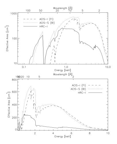
Figure 1.3: Comparison of the on-axis effective areas for observing a point source (integrated over PSF) of the **HRMA**/HRC-I, the **HRMA**/ACIS(FI), and the **HRMA**/ACIS(BI) combinations. The ACIS curves show the predicted values for the middle of Cycle 7 (2006-05-15).
