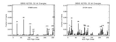
Figure 6.21: Fraction of ACIS background events as a function of grade from early in-flight data for an FI chip (S2) (left) and a BI chip (S3) (right).
