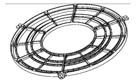
Figure 9.1: LETG Grating Element Support Structure, a machined aluminum plate approximately 110 cm in diameter which holds grating modules on a Rowland torus behind the *Chandra* mirrors.
