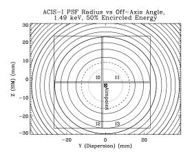
Figure 6.8: Approximate contours of constant 50% encircled energy at 1.49 keV when the ACIS-I default aimpoint is selected. The dotted line is 1 arcsec, the dashed line is 1.5 arcsec. The remainder are 1 arcsec intervals. The thicker solid lines highlight the 5, 10, and 15 arcsec contours.
