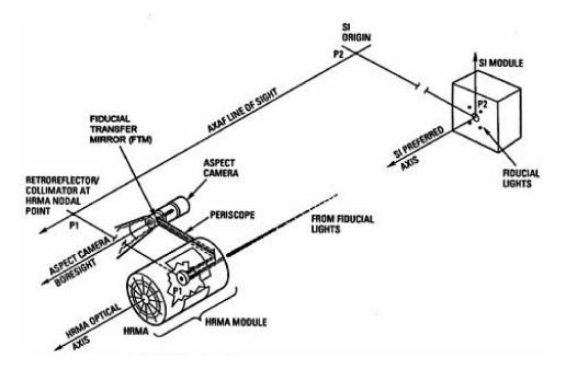
Figure 5.3: Fiducial Transfer System
