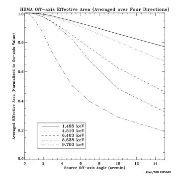
Figure 4.4: The **HRMA** effective area versus off-axis angle, averaged over azimuth, for selected energies, normalized to the on-axis area for that energy.
