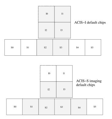
Figure 6.2: A schematic drawing of the ACIS focal plane, not to scale. The ACIS-I array consists of chips I0-I3. By default, chips I0-I3 plus S2 and S3 are turned on when ACIS-I is selected, as indicated in the top figure. ACIS-S consists of chips S0-S5. When operated in imaging mode chips S1-S4 plus I2 and I3 are turned on (bottom figure). When operated in spectroscopy mode S0-S5 are turned on.
