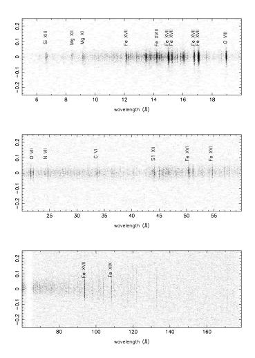
Figure 9.24: HRC-S detector image of a Capella observation, showing positive order dispersion. Both axes are in Å with 1.148 Å/mm. The increasing cross-dispersion extent of lines at longer wavelengths is due to astigmatism in the HRMA/LETG system. The positive-order HRC-S plate gap is at  $\sim 63$  Å.
