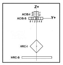
Figure 1.2: Arrangement of the ACIS and the HRC in the focal plane. The view is along the axis of the telescope from the direction of the mirrors. For reference, the two backilluminated ACIS-S chips are shaded. Numbers indicate positions of chips I0-I3 and S0-S5. SIM motion can be used to place the aimpoint at any point on the vertical solid line.
