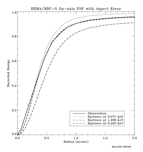
Figure 4.16: The fractional encircled energy as a function of angular radius observed in flight compared to model calculations for an on-axis point-source at selected X-ray energies. The curves are the combined response of the four nested mirror pairs, typical aspect uncertainties, and the HRC-S response function.
