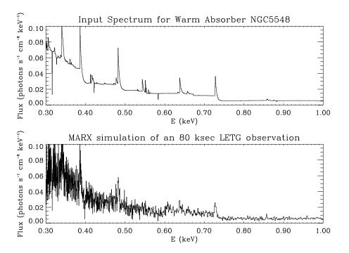
Figure 9.29: This figure shows the extracted first order spectrum for an 80 ksec observation of the AGN NGC5548. The input spectrum consists of a power–law plus a "warm" absorber (shown in the top panel). The simulated spectrum (bottom panel) has been corrected for the instrument response to give the flux from the source.
