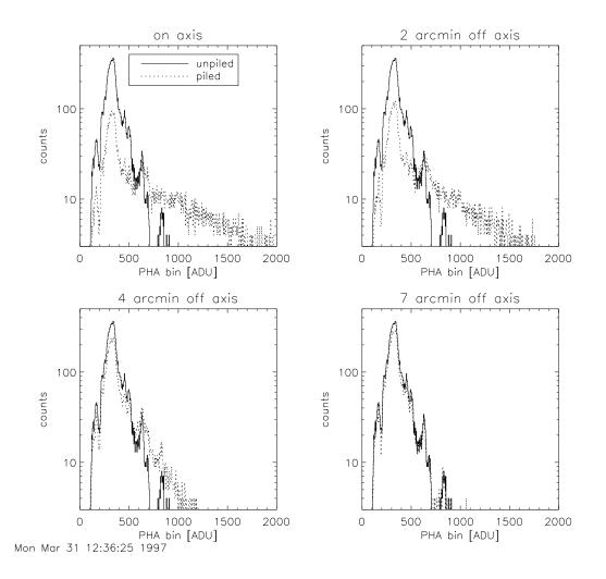
Figure 6.17: MARX simulations of the effect of pileup on the shape of the spectrum. The true (solid line) and the detected (dotted line) spectra are shown for four different viewing angles. The corresponding "pileup fractions" - see Section 6.14.2 - are 46%, 40%, 15%, and 2% as the image is moved progressively further off-axis. (Source: J. Kastner and M. Wise, CXC)
