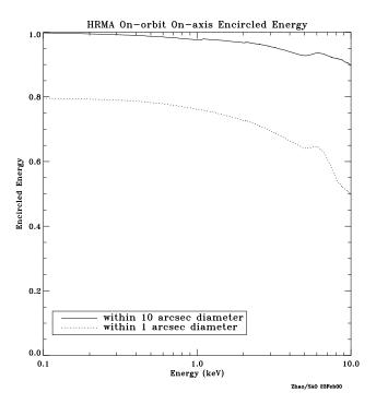
Figure 4.7: On-orbit performance prediction for encircled energy, calculated from model derived from ground-based calibration data.
