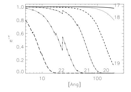
Figure 9.27: The ISM transmittance within the LETGS bandpass for different values of neutral hydrogen column density  $10^{17}$ - $10^{22}$  cm<sup>2</sup>.
