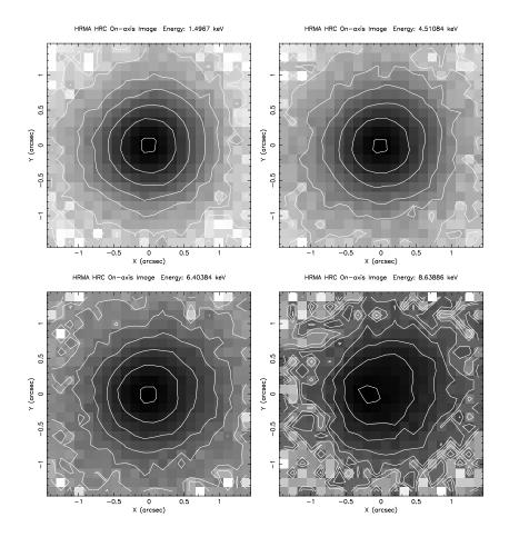
Figure 4.10: Simulated on-axis **HRMA**/HRC-I on-axis images of mono-energetic point sources without aspect blurring. Energies are 1.49, 4.51, 6.40, and 8.63 keV. Surface brightness contours are logarithmic and spaced in factors of 3. The innermost contour is at 90% of the peak brightness. The 8.6 keV image core is off-center due to the shell 6 misalignment. Each panel is 3" square.
