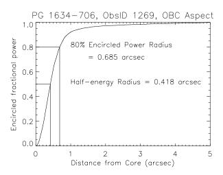
Figure 6.7: The on-orbit encircled broad-band energy versus radius for an ACIS observation of point source PG1634-706. The effective energy is 1 keV.
