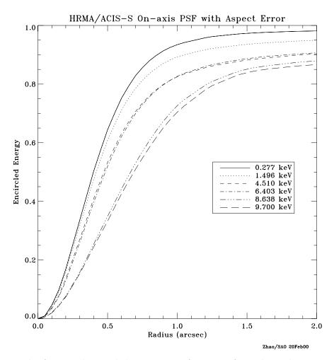
Figure 4.15: The fractional encircled energy as a function of angular radius expected for in flight ACIS-S(S3) measurements for an on-axis point-source at selected X-ray energies. The curves are the combined response of the four nested mirror pairs, typical aspect uncertainties, and the ACIS response function.
