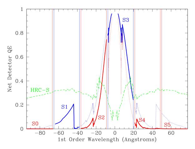
Figure 9.6: (Y-offset = 0 for HRC-S, -0.33' for ACIS-S). Dashed (green) line is for HRC-S, thick solid curves are for ACIS (updated for AO6 QE degradation). Y-offsets may be chosen to tailor the coverage of BI chips (S1 and S3; top/blue QE curve) and FI chips (S0,S2,S4,S5; bottom/red curve). Vertical lines indicate ACIS chip gaps (with dither, 1.5 Å). For clarity, -3 to +3 Å is not shown for ACIS.
