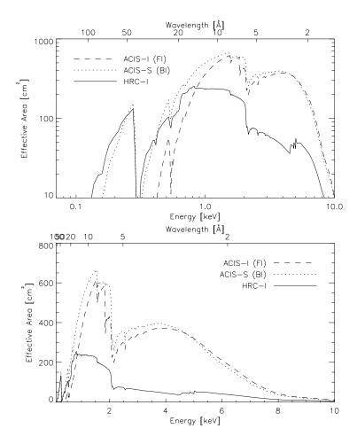
Figure 1.3: Comparison of the on-axis effective areas for observing a point source (integrated over PSF) of the HRMA/HRC-I, the HRMA/ACIS(FI), and the HRMA/ACIS(BI) combinations. The ACIS curves show the predicted values for the middle of Cycle 6 (2005-05-15).
