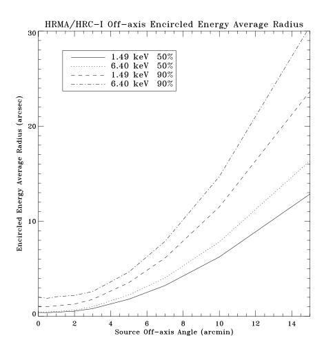
Figure 4.9: HRMA/HRC-I encircled energy average radii for circles enclosing 50% and 90% of the power at 1.49 and 6.40 keV as a function of off-axis angle. The HRC-I surface is a flat plane perpendicular to the optical axis, which does not follow the curved Chandra focal plane. These curves include the blurs due to the HRC-I spatial resolution and the Chandra aspect error.
