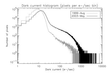
Figure 5.5: Differential histogram of dark current distribution for the ACA CCD in 1999-Aug (gray) and 2003-Apr (black)
