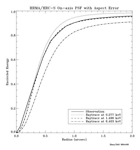
Figure 4.14: The fractional encircled energy as a function of angular radius observed in flight compared to model calculations for an on-axis point-source at selected X-ray energies. The curves are the combined response of the four nested mirror pairs, typical aspect uncertainties, and the HRC-S response function.
