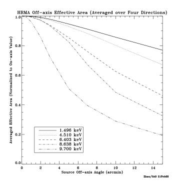
Figure 4.4: The HRMA effective area versus off-axis angle, averaged over azimuth, for selected energies, normalized to the on-axis area for that energy.
