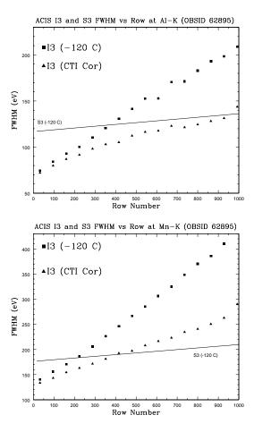
Figure 6.12: An example of the application of the CXC CTI-corrector in two energy bands. The first plot shows data for the Al-K line, and the second for Mn-K. The square data points are the FWHM of lines accumulated in 32-row bins. The triangle data points are the FWHM of CTI-corrected lines accumulated in 32-row bins. The line shows the nominal performance of the S3 chip. This data is from March 2000.
