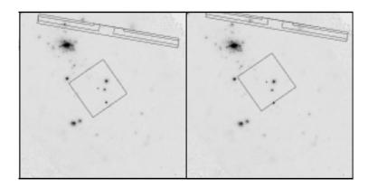
Figure 3.2: Example of offset pointing with HRC. North is up and East is to the left. Roll is measured positive, West of North. The roll angle shown is 10°. Left Panel: The target, the middle source in a group of three aligned N-S, is offset from the HRC-I nominal aimpoint with (Y,Z) offset of (-5,0) arcmin. Right Panel: The offset is (-5,-5). Note the small dot at the location of the HRC-I aimpoint.
