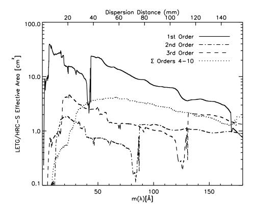
Figure 9.18: The combined HRMA/LETG/HRC-S effective area, illustrating the relative strengths of 1st and higher orders. Positive and negative orders are summed. In the label for the bottom axis, m is the order number. See the text for an example of how to determine the relative strength of overlapping lines from different orders.
