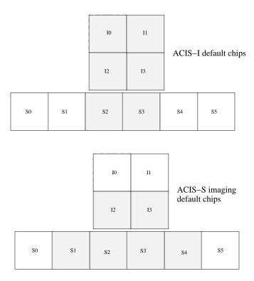
Figure 6.2: A schematic drawing of the ACIS focal plane, not to scale. The ACIS-I array consists of chips I0-I3. By default, chips I0-I3 plus S2 and S3 are turned on when ACIS-I is selected, as indicated in the top figure. ACIS-S consists of chips S0-S5. When operated in imaging mode chips S1-S4 plus I2 and I3 are turned on (bottom figure). When operated in spectroscopy mode S0-S6 are turned on.
