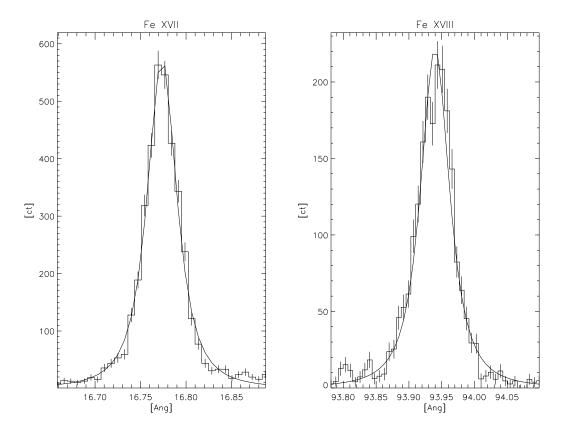
Figure 9.9: LETGS line response function as illustrated by two bright Fe lines (Fe XVII at  $\sim 17$  Å and Fe XVIII at  $\sim 94$  Å) using in-flight calibration observations of Capella. The solid curves are best fit beta models ( $\beta = 2.5$ ).
