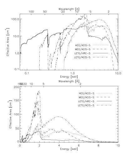
Figure 1.4: Comparison of the first-order effective areas in  $\rm cm^2$  (integrated over the line spread function) of the MEG and HEG and LETG spectrometers. The (+/-) first orders of the diffracted spectrum have been added.
