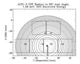
Figure 6.9: Approximate contours of constant 50% encircled energy at 1.49 keV when the ACIS-S default aimpoint is selected. The dotted line is 1 arcsec, the dashed line is 1.5 arcsec. The remainder are 1 arcsec intervals. The thicker solid lines highlight the 5, 10, 15 and 20 arcsec contours.
