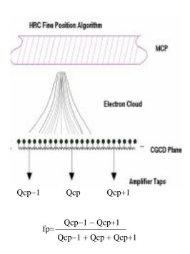
Figure 7.4: Schematic representation of event position determination for one axis of the crossed grid charge detector (CGCD). The electron cloud is divided between several amplifiers. The position of the event relative to the central coarse position is calculated from the difference between the signals on either side of the coarse position divided by the sum of the three signals.
