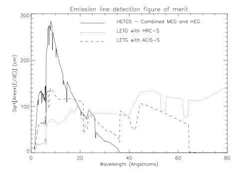
Figure 8.28: The figure of merit for detecting isolated emission lines computed according to the equations in Section 8.5.4 for the HETGS, LETG with HRC-S and for the LETG with ACIS-S. The results indicate that the LETG with the HRC-S is preferred if the emission lines of interest have wavelengths longer than 20 Å (or  $0.62~\rm keV$ ) while the HETGS is best for emission lines shorter than about 16 Å (or  $0.78~\rm keV$ ).
