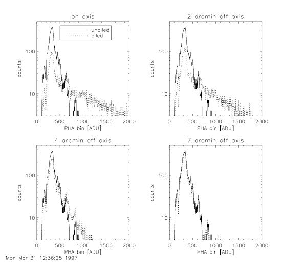
Figure 6.13: MARX simulations of the effect of pileup on the shape of the spectrum. The true (solid line) and the detected (dotted line) spectra are shown for four different viewing angles. The corresponding "pileup fractions" - see Section 6.14.2 - are 46%, 40%, 15%, and 2% as the image is moved progressively further off-axis. (Source: J. Kastner and M. Wise, CXC)
