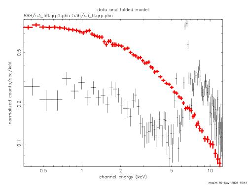
Figure 6.26: Spectra of different background flares in chip S3. Thick crosses show a common flare species that affects only the BI chips. Thin crosses show one of the several less common flare species that affect both the BI and FI chips. Note how both these spectra are different from the quiescent spectrum (see Figure 6.23).
