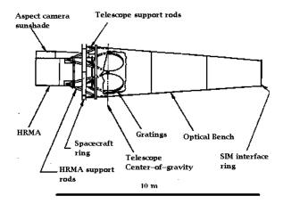
Figure 2.1: Major components of the telescope system.
