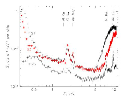
Figure 6.21: Energy spectra of the charged particle ACIS background (standard grade filtering) with ACIS in the stowed position taken in 2002, September. Line features are due to fluorescence of material in the telescope and focal plane.
