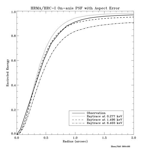
Figure 4.13: The fractional encircled energy as a function of angular radius observed in flight compared to model calculations for an on-axis point-source at selected X-ray energies. The curves are the combined response of the four nested mirror pairs, typical aspect uncertainties, and the HRC-I response function.
