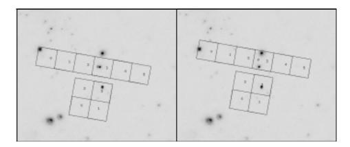
Figure 3.1: Examples of offset pointing with ACIS. North is up and East is to the left. Roll is measured positive, West of North. The roll angle shown is 10°. Left Panel: The target, a bright x-ray source, is offset from the ACIS-S nominal aimpoint with (Y,Z) offset of (-1,0) arcmin. In the Right Panel the offset is (-1,-3). Note the small circle at the location of the ACIS-S aimpoint.
