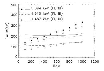
Figure 6.11: The energy resolution of S3 and I3 as a function of row number. These data were taken at  $-120^{\circ}$ C. Note that these curves are representative of the variation - but they do not account for the row-dependent gain variation which also increases the energy resolution by about 10-15%, especially for the larger row numbers.
