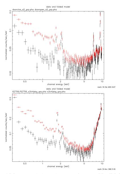
Figure 6.23: ACIS quiescent background spectrum for an FI CCD (S2) (top) and a BI CCD (S3)(bottom). The lower curve shows the spectrum before the HRMA doors were opened; the upper curve after. Both curves have G02346 filtering.
