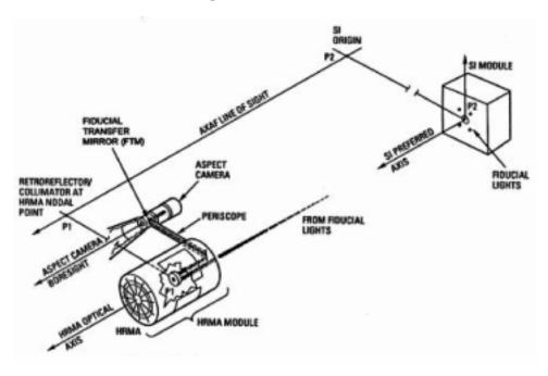
Figure 5.3: Fiducial Transfer System
