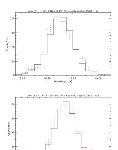
Figure 8.17: Representative Line Response Functions at two wavelengths for the MEG; 19 Å top, 6.7 Å bottom. Two of the bright lines in the MEG Capella spectrum shown in Figure 8.2 have been fit by the instrumental LRF. The LRF is encoded in the MEG RMF created using CXC software and calibration parameters (mkgrmf, lsfparmN0003.)
