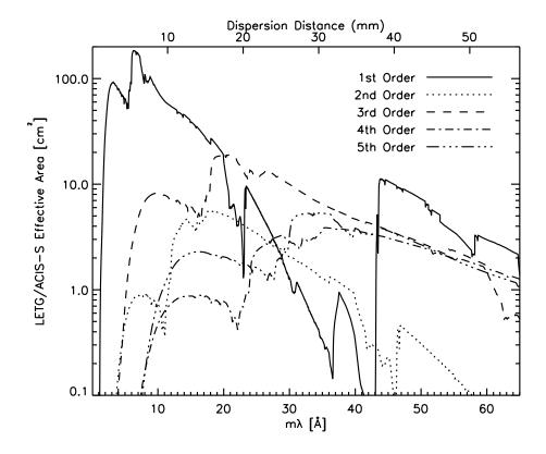
Figure 9.20: The combined HRMA/LETG/ACIS-S effective areas for first and higher orders. LETG+ACIS-S areas were computed using an effective area model that included the effects of contamination build-up extrapolated to the level expected in mid-May 2005. Positive and negative orders are summed.
