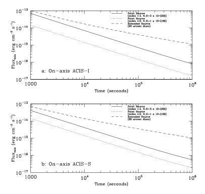
Figure 6.27: The minimum detectable flux as a function of exposure time for an on-axis observation of a point source using an FI chip (top) and a BI chip (bottom). The calculation assumes a  $3\sigma$  2-10 keV absorbed flux detection criterion in a 5x5 pixel detection cell and no pileup. The power law index is a photon index. The extended source spectrum assumed the -1.4 index power law and corresponding column.
