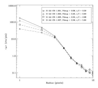
Figure 6.18: The effects of pileup on the radial distribution of the PSF are illustrated. These data were taken during ground calibration at the XRCF. The specific "OBSIDs", the counting rate per CCD frame ("c/f"), and the "pileup fraction" as defined in Section 6.14.2 are given in the inset.
