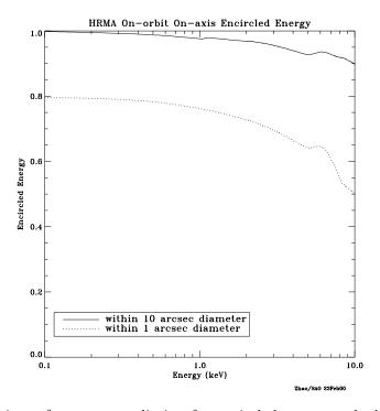
Figure 4.7: On-orbit performance prediction for encircled energy, calculated from model derived from ground-based calibration data.
