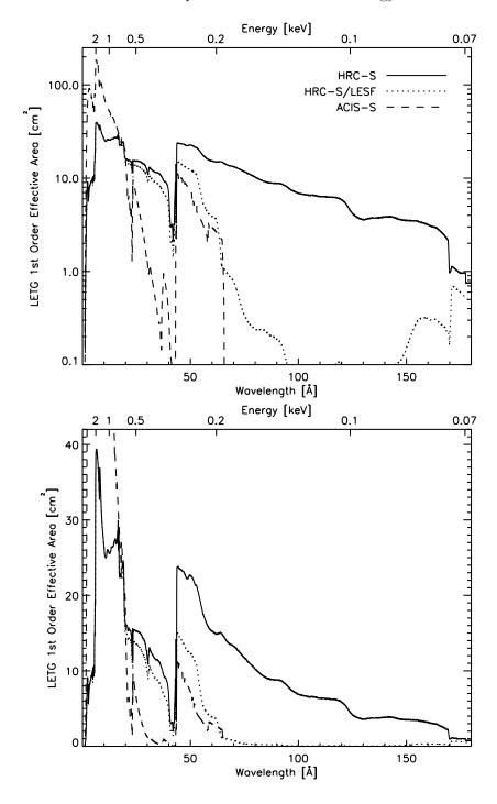
Figure 9.17: LETGS 1st-order effective area for an on-axis point source, with HRC-S, HRC-S LESF and ACIS-S detector configurations with log and linear scaling. Positive and negative orders summed. LETG+ACIS-S areas were computed using an effective area model that included the effects of contamination build-up extrapolated to the level expected in mid-May 2005. Note that the vertical scale of the linear plot has been truncated.
