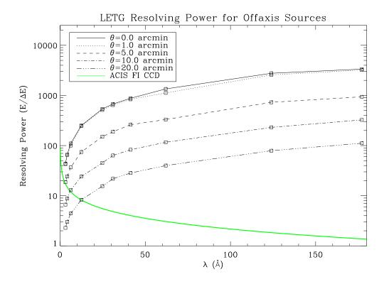
Figure 9.12: LETG spectral resolving power for off-axis sources. The predicted LETG resolving power ( $\rm E/\Delta E$ ) is shown versus wavelength for various off-axis distances. The MARX simulator has been used, which somewhat overestimates the on-axis resolving power. For comparison, the spectral resolution for ACIS front-illuminated CCD chips is shown. Note that the ACIS/FI curve does not include the effects of CTI, which progressivly degrades resolution away from the readout edge.
