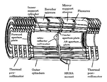
Figure 4.1: The 4 nested HRMA mirror pairs and associated structures.
