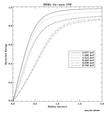
Figure 4.6: The fractional encircled energy as a function of angular radius calculated for an on-axis point-source, at selected X-ray energies. The curves are the combined response of the four nested mirror pairs.
