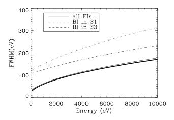
Figure 6.10: The ACIS pre-launch energy resolution as a function of energy. (Source: CXC Calibration group).
