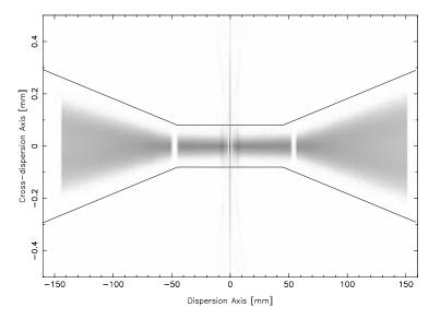
Figure 9.14: A MARX simulation of a flat spectrum illustrating the broadening of the LETG+HRC-S profile in the cross-dispersion direction, and showing the "bow-tie" spectral extraction window.
