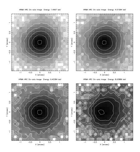
Figure 4.8: Simulated on-axis HRMA/HRC-I on-axis images of mono-energetic point sources without aspect blurring. Energies are 1.49, 4.51, 6.40, and 8.63 keV. Surface brightness contours are logarithmic and spaced in factors of 3. The innermost contour is at 90% of the peak brightness. The 8.6 keV image core is off-center due to the shell 6 misalignment. Each panel is 3'' square.
