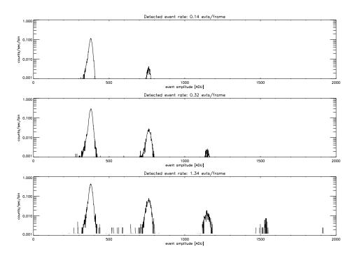
Figure 6.17: The effects of pileup at 1.49 keV (Al K $\alpha$ ) as a function of source intensity. Data were taken during HRMA-ACIS system level calibration at the XRCF. Single-photon events are concentrated near the pulse height corresponding to the Al K $\alpha$  line ( $\sim 380$  ADU), and events with 2 or more photons appear at integral multiples of the line energy.
