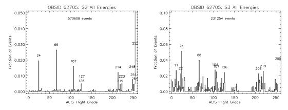
Figure 6.22: Fraction of ACIS background events as a function of grade from early in-flight data for an FI chip (S2) (left) and a BI chip (S3) (right).
