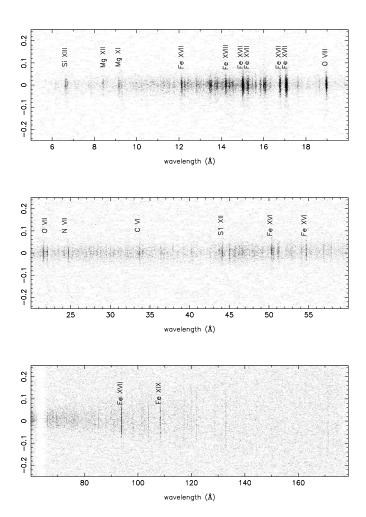
Figure 9.25: HRC-S detector image of a Capella observation, showing positive order dispersion. Both axes are in Å with 1.148 Å/mm. The increasing cross-dispersion extent of lines at longer wavelengths is due to astigmatism in the HRMA/LETG system. The positive-order HRC-S plate gap is at  $\sim 63$  Å.
