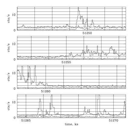
Figure 6.27: An example of the ACIS background counting rate versus time - BI chip (S3; top curve) and an FI chip (I2; bottom curve). These are for the standard grades and the band from 0.3 -  $10~\rm keV$ .
