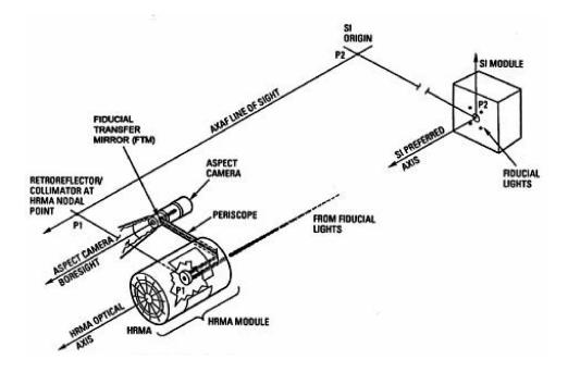
Figure 5.3: Fiducial Transfer System
