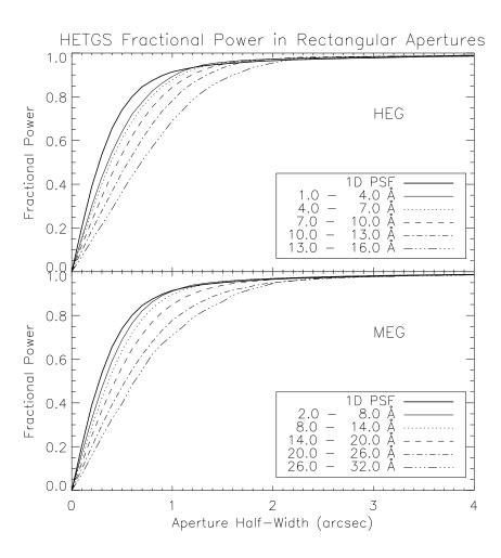
Figure 8.22: Enclosed power distributions are computed for five wavelength intervals for both the HEG (top) and the MEG (bottom). The observation of Mk 421 (observation ID 1714) was used.
