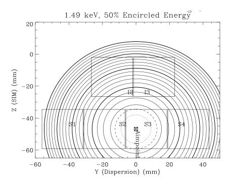
Figure 6.12: Approximate contours of constant 50% encircled energy at 1.49 keV when the ACIS-S default aimpoint is selected. The dotted line is 1 arcsec, the dashed line is 1.5 arcsec. The remainder are at 1 arcsec intervals. The thicker solid lines highlight the 5, 10, 15 and 20 arcsec contours.
