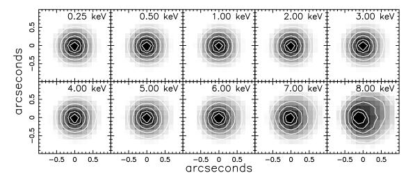
Figure 4.8: Simulated on-axis HRMA/HRC-I images of on-axis mono-energetic point sources with aspect blurring. The grayscale is a linear stretch; surface brightness contours are at 90%, 80%, 60%, 40%, and 20% of the peak brightness. The 8 keV image core is asymmetric and off-center due to the shell 6 misalignment.
