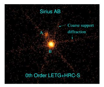
Figure 9.27: LETG/HRC-S zeroth order image of Sirius A and B. The two stars are separated by  $\sim 4''$ . Flux from Sirius A is due to the small but finite UV response of the detector. The star-shaped structure is due to coarse support diffraction.
