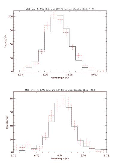
Figure 8.17: Representative Line Response Functions at two wavelengths for the MEG; 19 Å top, 6.7 Å bottom. Two of the bright lines in the MEG Capella spectrum shown in Figure 8.2 have been fit by the instrumental LRF. The LRF is encoded in the MEG RMF created using CXC software and calibration parameters.
