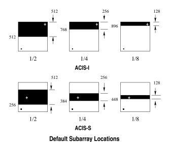
Figure 6.15: Examples of various subarrays. The heavy dot in the lower left indicates the origin
