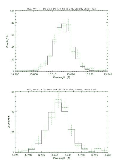
Figure 8.16: Representative Line Response Functions at two wavelengths for the HEG; 15 Å top, 6.7 Å bottom. Two of the bright lines in the HEG counterpart to the MEG Capella spectrum shown in Figure 8.2 have been fit by the instrumental LRF. The LRF is encoded in the HEG RMF created using CXC software and calibration parameters.
