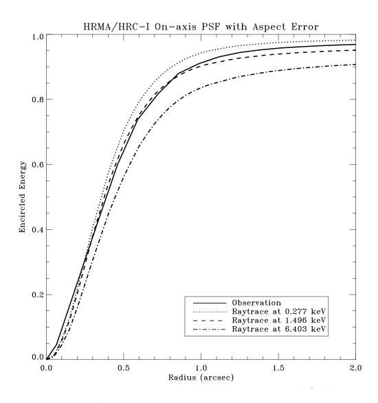
Figure 4.21: The HRMA/HRC-I on-axis fractional encircled energy as a function of angular radius from a point source (Ar Lac) observed in flight compared to ray trace simulations for an on-axis point-source at selected X-ray energies, including the aspect uncertainties and the HRC-I pixelization effects.
