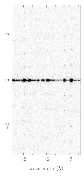
Figure 9.24: Detail of Figure 9.23, showing the LETG/HRC-S image of bright lines in Capella. Both axes are in Å with 1.148 Å/mm. The Fe XVII lines at  $\sim 15$  and 17 Å are the brightest in the LETG Capella spectrum. Faint features above and below the primary spectrum are due to fine support structure diffraction.
