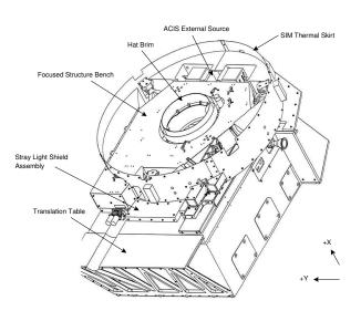
Figure 2.1: A schematic of the Science Instrument Module.
