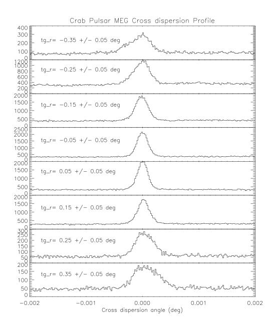
Figure 8.20: The cross dispersion profile is shown for eight slices of the dispersed MEG spectrum of the Crab pulsar. There is an asymmetry caused by misaligned gratings that becomes most evident at large dispersion.
