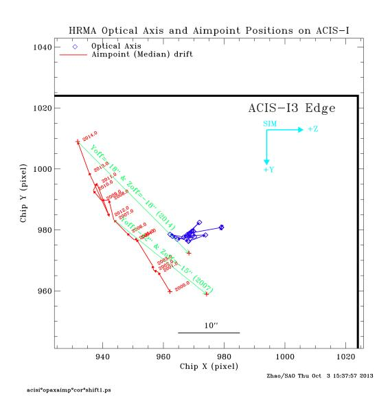
Figure 6.14: Positions of the optical axis and aimpoint on the I3 CCD at various times in the mission. Since 1999, the aimpoint (position of optimal focus) has drifted (dark lines), and default pointing offsets (lighter lines) have been changed several times to move the image away from the edge of the chip. All dates in red refer to the beginning of the given year.
