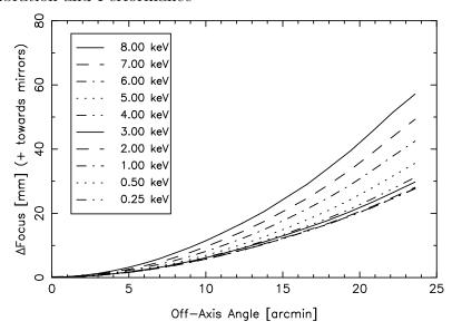
Figure 4.11: The HRMA focal surface (from simulations), indicating its dependence on energy and off-axis source position.
