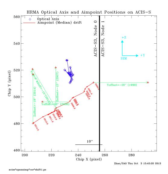
Figure 6.13: Positions of the optical axis and aimpoint on the S3 CCD at various times in the mission. Since 1999, the aimpoint (position of optimal focus) has drifted (dark lines), and default pointing offsets (lighter lines) have been changed several times to move the image away from the node boundary. All dates in red refer to the beginning of the given year.
