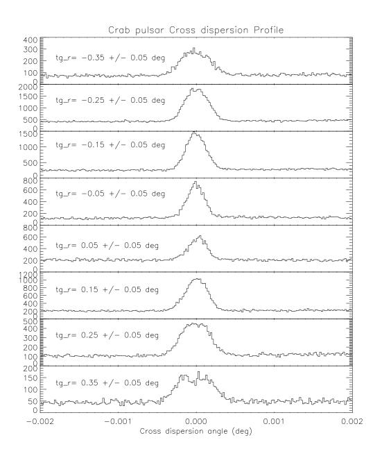
Figure 8.21: As in Figure 8.21, the cross dispersion profile is shown for the HEG spectrum of the Crab pulsar. The profile is symmetric but broadens significantly at large dispersion.
