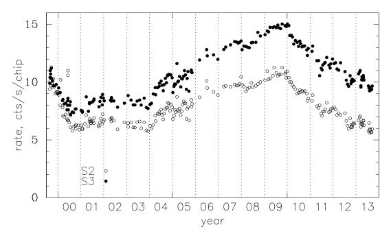
Figure 6.26: Total telemetered background rates (including all grades and the upper event cutoff at 15 keV) for chips S2 (FI) and S3 (BI) as a function of time. Vertical dashed lines are year boundaries.
