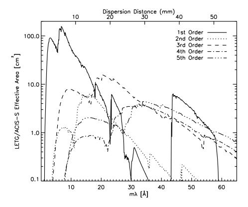
Figure 9.20: The combined HRMA/LETG/ACIS-S effective areas for 1st and higher orders. LETG+ACIS-S areas were computed using an effective area model that included the effects of contamination build-up extrapolated to the level expected in mid-2015. Positive and negative orders are summed.
