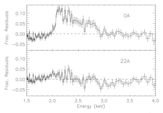
Figure 4.2: Combined residuals from power-law fits to 18 blazar observations (Marshall, H.L., 2005). The residuals in the upper panel are based upon models of contaminant free optics, while those in the lower are based upon a model of the mirror surfaces which includes a thin (22Å) hydrocarbon layer.
