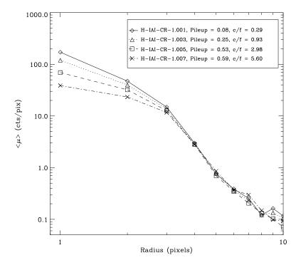
Figure 6.19: The effects of pileup on the radial distribution of the PSF are illustrated. These data were taken during ground calibration at the XRCF. The specific "OBSIDs", the counting rate per CCD frame ("c/f"), and the "pileup fraction" as defined in Section 6.15.2 are given in the inset.
