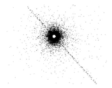
Figure 6.16: Trailed image of a strong X-ray source. The core of the image is faint due to pileup. Most events here are rejected because of bad grades. The readout direction is parallel to the trail.
