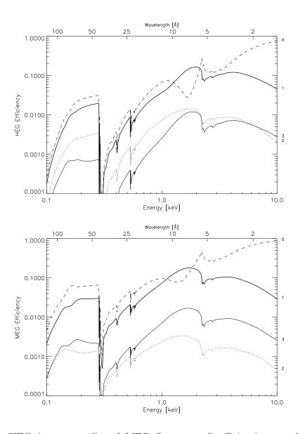
Figure 8.13: HEG (upper panel) and MEG (lower panel) efficiencies as a function of energy. The values plotted are the mirror-weighted efficiency into a single plus, minus, or zero order (labelled on the right edge). The dashed line is zeroth order; the thick solid line is first order. Note that the relative strengths of the third orders (thin solid lines) are comparable, whereas the second order strengths (dotted lines) are significantly different between the HEG and MEG.
