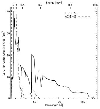
Figure 9.17: LETGS 1st-order effective area for an on-axis point source, with HRC-S and ACIS-S detector configurations with log (top) and linear (bottom) scaling. Positive and negative orders are summed. LETG+ACIS-S areas were computed using an effective area model that included the effects of contamination build-up extrapolated to the level expected in mid-2015. Note that the vertical scale of the linear plot has been truncated.
