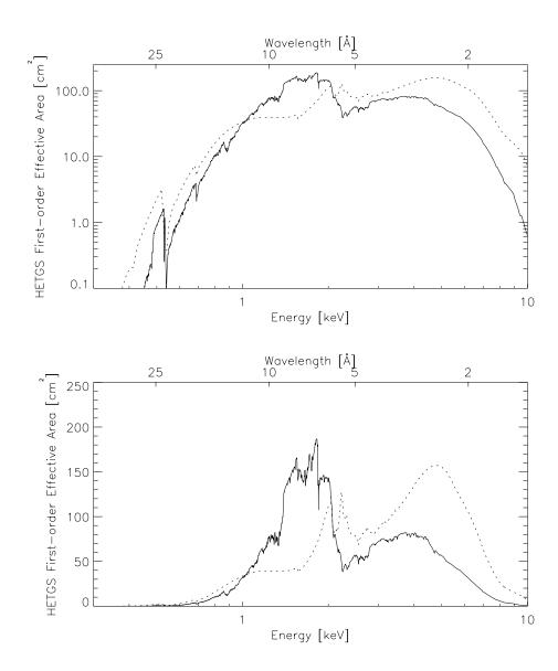
Figure 8.11: The modeled total first-order (solid curve) and zeroth-order (dotted curve) effective area, integrated over the PSF, of the  $\mathbf{HRMA}$ -HETG-ACIS-S combination, as a function of energy. The first-order data are the same as those plotted in Figures 8.7 and 8.9. The plotted first-order values are the sums of the area at a particular energy from both orders (+/-) of both MEG and HEG spectra. Both a log-log and a log-linear version are shown.
