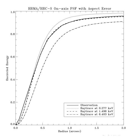
Figure 4.22: The HRMA/HRC-S on-axis fractional encircled energy as a function of angular radius from a point source (LMC X-1) observed in flight compared to ray trace simulations for an on-axis point-source at selected X-ray energies, including the aspect uncertainties and the HRC-S pixelization effects.
