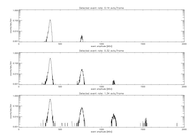
Figure 6.18: The effects of pileup at 1.49 keV (Al K $\alpha$ ) as a function of source intensity. Data were taken during HRMA-ACIS system level calibration at the XRCF. Single-photon events are concentrated near the pulse height corresponding to the Al K $\alpha$  line ( $\sim$  380 ADU), and events with 2 or more photons appear at integral multiples of the line energy.
