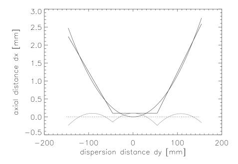
Figure 9.5: The front surfaces of the HRC-S detector segments and their relationship to the Rowland circle are shown schematically. The scalloped line beneath them is the difference between the detector surface and the Rowland circle.
