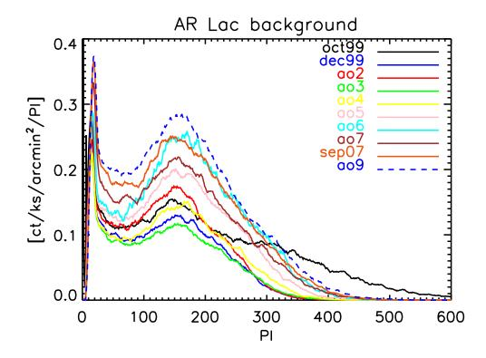
Figure 7.17: Average background spectra in the inner 10' region of the detector, obtained from yearly observations towards AR Lac are shown. Times of high background flaring have been excluded. The magnitude and shape of the spectra vary considerably with time, but may be interpolated between epochs to estimate the background for any given observation.
