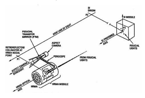
Figure 5.3: Fiducial Transfer System
