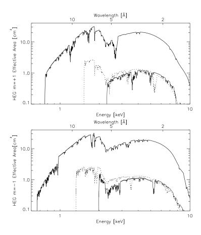
Figure 8.7: The HETGS HEG effective area, integrated over the PSF, is shown with energy and wavelength scales. The m=+1,+2,+3 orders (falling on ACIS chips S5, S4, S3; left to right) are displayed in the top panel and the m=-1,-2,-3 orders (falling on ACIS chips S0, S1, S2; left to right) are in the bottom panel. The thick solid lines are first order; the thin solid line is third order; and the dotted line is second order.
