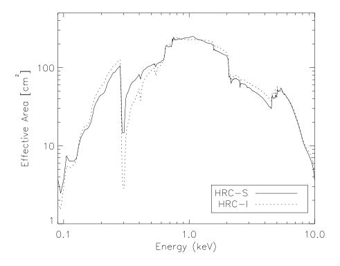
Figure 7.15: The effective area of the HRMA/HRC-I (dashed line) and the central segment of the HRMA/HRC-S in imaging mode (solid line) integrated over the full PSF. Absorption edges are due to the iridium coating on the mirrors, the CsI MCP coating, and the polyimide/Al of the UVIS.
