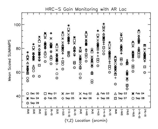
Figure 7.13: As in Figure 7.12, for the HRC-S. The mean scaled SUMAMPS decline with time at all pointings, as is seen for the HRC-I in Figure 7.12. A time dependent gain correction can be applied to normalize the scaled SUMAMPS such that 1 keV photons are centered at PI=128.
