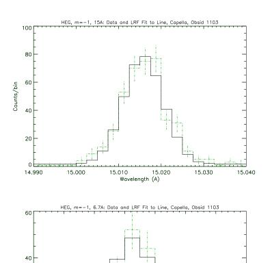
Figure 8.15: Representative Line Response Functions at two wavelengths for the HEG; 15 Å top, 6.7 Å bottom. Two of the bright lines in the HEG counterpart to the MEG Capella spectrum shown in Figure 8.2 have been fit by the instrumental LRF. The LRF is encoded in the HEG RMF created using CXC software and calibration parameters.
