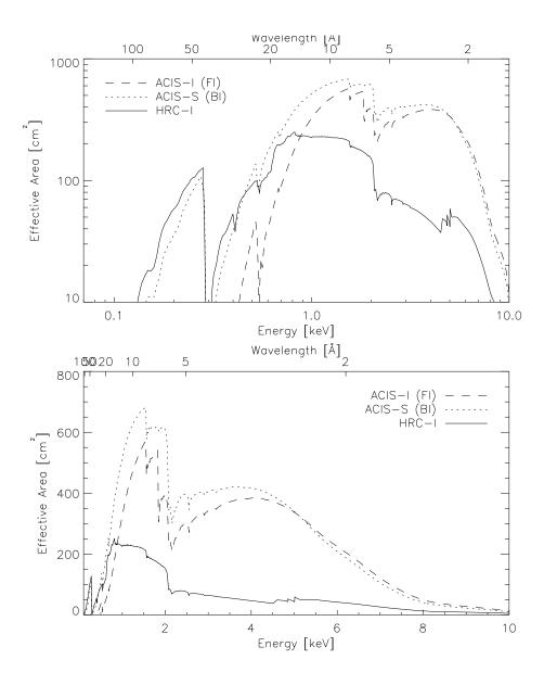
Figure 1.3: Comparison of the on-axis effective areas for observing a point sourc(integrated over the PSF) of the HRMAHRC-I, the HRMA/ACIS(FI), and the HRMA/ACIS(BI) combinations. The ACIS curves show the predicted values for the middle of Cycle 12 (2010-05-15).
