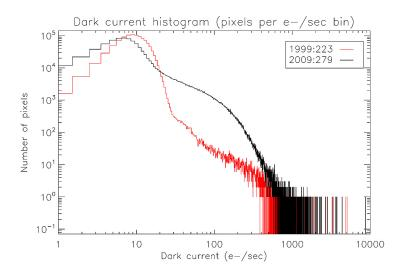
Figure 5.6: Differential histogram of dark current distribution for the ACA CCD in 1999-Aug and 2009-Oct
