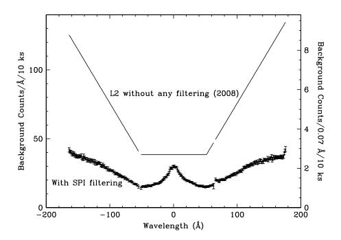
Figure 9.21: The LETG+HRC-S background rate with and without the new SPI filter. Data are shown using the standard 'bowtie' spectral extraction region (see Figure 9.14). X-ray losses from the observed spectrum as a result of the filtering for 1st order are ~1.25%; losses will be slightly higher for higher orders. See http://cxc.harvard.edu/cal/Letg/Hrc\_bg for more information.
