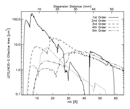
Figure 9.20: The combined HRMA/LETG/ACIS-S effective areas for 1st and higher orders. LETG+ACIS-S areas were computed using an effective area model that included the effects of contamination build-up extrapolated to the level expected in mid-May 2010. Positive and negative orders are summed.
