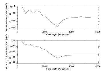
Figure 7.14: The HRC-I (top) and the center section of the HRC-S (bottom) UV/Ion shield effective area as a function of wavelength.
