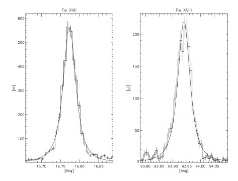
Figure 9.9: LETGS line response function as illustrated by two bright Fe lines (Fe XVII at  $\sim 17$  Å and Fe XVIII at  $\sim 94$  Å) using in-flight calibration observations of Capella. The solid curves are best-fit Moffat functions with  $\beta=2.5$ .
