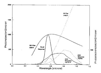
Figure 5.2: Spectral response of the ACA CCD. The same signal-to-noise is achieved for a V=11.7 magnitude N0 star as for a V=10 magnitude G0V star. Also shown are the spectra and the standard visual response for the two stars.
