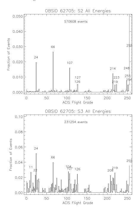
Figure 6.22: Fraction of ACIS background events as a function of grade from early in-flight data for an FI chip (S2) (left) and a BI chip (S3) (right).
