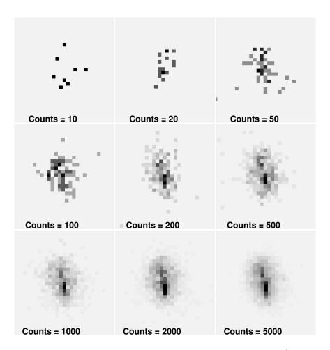
Figure 4.16: A simulated 1.49 keV point source at an off-axis angle of 5', binned to ACIS pixels. The panels show what the source would look like with a varying number of counts. Note how the apparent morphology is a strong function of the number of counts, and how even with a large number of counts one might mistake it for an extended source or even for multiple sources.
