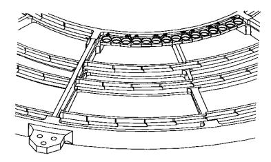
Figure 9.2: Detail of the LETG Grating Element Support Structure showing grating modules mounted on the inner annulus.
