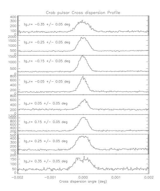
Figure 8.20: As in Figure 8.20, the cross dispersion profile is shown for the HEG spectrum of the Crab pulsar. The profile is symmetric but broadens significantly at large dispersion.
