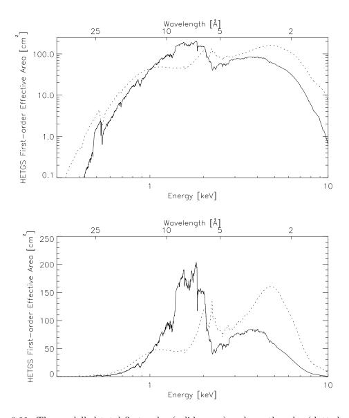
Figure 8.11: The modelled total first-order (solid curve) and zeroth-order (dotted curve) effective area, integrated over the PSF, of the  $\mathbf{HRMA}$ -HETG-ACIS-S combination, as a function of energy. The first-order data are the same as those plotted in Figures 8.7 and 8.9. The plotted first-order values are the sums of the area at a particular energy from both orders (+/-) of both MEG and HEG spectra. Both a log-log and a log-linear version are shown.
