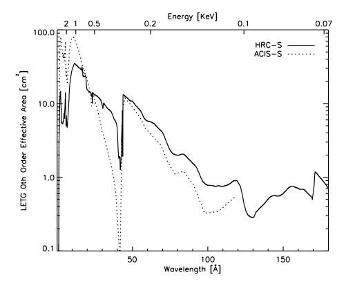
Figure 9.16: LETGS zeroth-order effective area for an on-axis point source for the LETG with HRC-S and ACIS-S detectors. The zeroth-order effective area for the HRC-S/LESF combination is the same as for the HRC-S. LETG+ACIS-S areas were computed using an effective area model that included the effects of contamination build-up extrapolated to the level expected in mid-May 2010.
