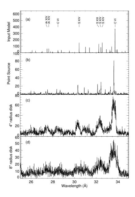
Figure 9.29: MARX simulation of spectra showing the effect of source extent. The panels show (a) computed input spectrum, (b) a MARX output of LETG spectrum of a point source, (c) the same as (b) except that the source is a disc of uniform brightness with radius of 4'', and (d) the same but with radius of 8''. See Figure 9.11 and Section 9.3.3 for a discussion of extended sources.
