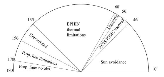
Figure 3.4: Diagram to illustrate ranges of solar pitch angle (the angle between the pointing direction and the satellite-Sun line) within which different observing limitations apply. Table 3.1 provides quantitative estimates for the observing limitations in the solar pitch angle ranges shown in the drawing.
