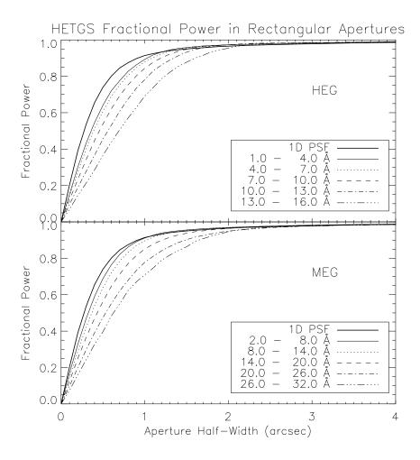
Figure 8.21: Enclosed power distributions are computed for five wavelength intervals for both the HEG (top) and the MEG (bottom). The observation of Mk 421 (observation ID 1714) was used.
