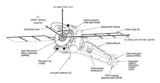
Figure 1.1: The *Chandra* Observatory with certain subsystems labeled.
