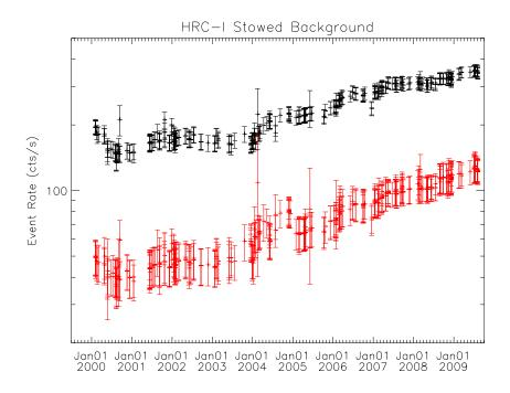
Figure 7.18: The change in HRC-I stowed background rate with time. The total rate (black points and error bars, upper set) and the valid rate (red points and error bars, lower set) are shown. The HRC-S data are similar.
