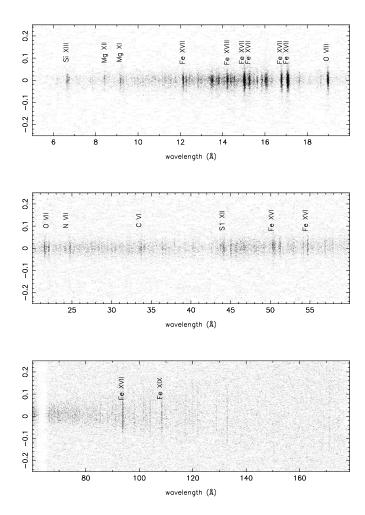
Figure 9.24: HRC-S detector image of a Capella observation, showing positive order dispersion. Both axes are in Å with 1.148 Å/mm. The increasing cross-dispersion extent of lines at longer wavelengths is due to a stigmatism in the HRMA/LETG system. The positive-order HRC-S plate gap is at  $\sim63~\textrm{Å}.$
