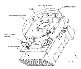
Figure 2.2: A schematic of the Science Instrument Module.
