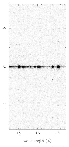
Figure 9.23: Detail of Figure 9.22, showing the LETG/HRC-S image of bright lines in Capella. Both axes are in Å with 1.148 Å/mm. The Fe XVII lines at  $\sim 15$  and 17 Å are the brightest in the LETG Capella spectrum. Faint features above and below the primary spectrum are due to fine support structure diffraction.
