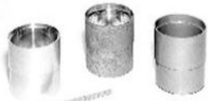
3 inch diameter solar X-ray telescope mirrors
